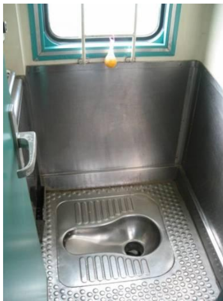
Figure 2.48 Stainless Steel Squat Toilets ("Beijing venues," (n.d.))
