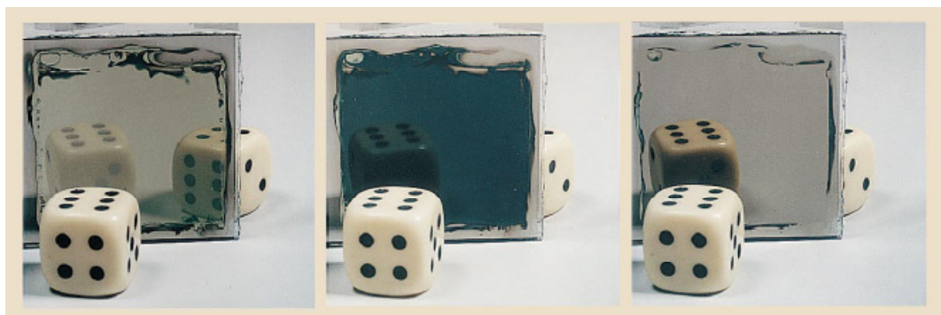
Figure 2.6 Transparent, dark and reflective states of a Gd 30 Mg 70 alloy. The states can be switched by pumping hydrogen in and out of a cell that contains the alloy film. (Ball, 1998)
