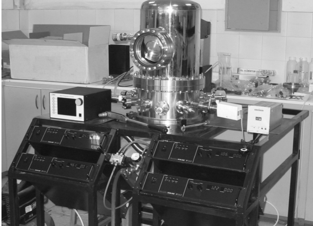
Figure 3.1 The custom-made thermal evaporation unit. (Akyıldız, 2009)
