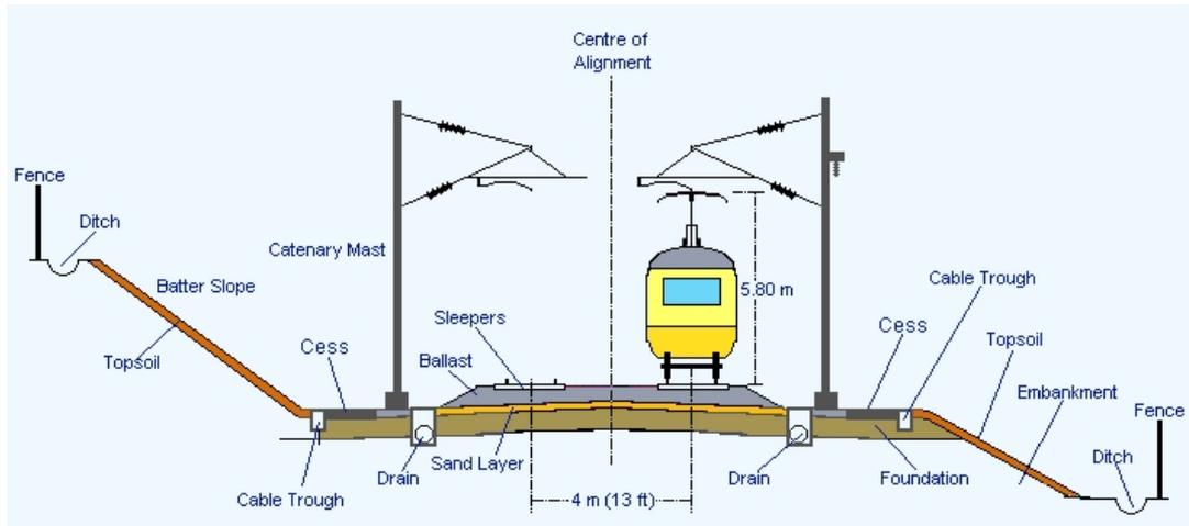
Figure 4.1: Typical cross section of double track railway
