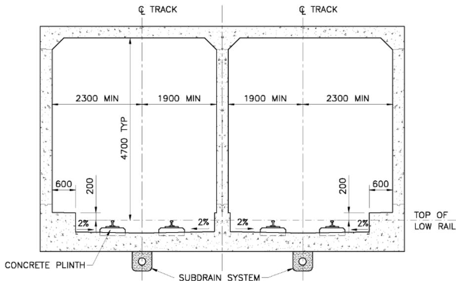
Figure 4.4: Cross-section of direct fixation trackway on tunnel
