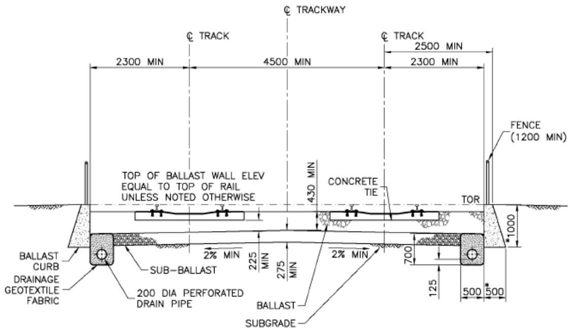
Figure 4.3: A detailed cross-section of ballasted trackway
