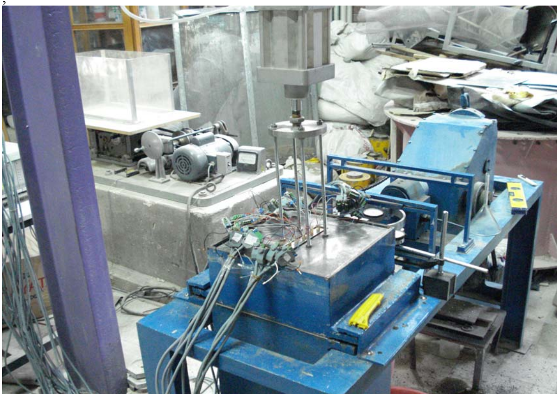
Figure 3.21 Cable Connection in Group Pile Tests
