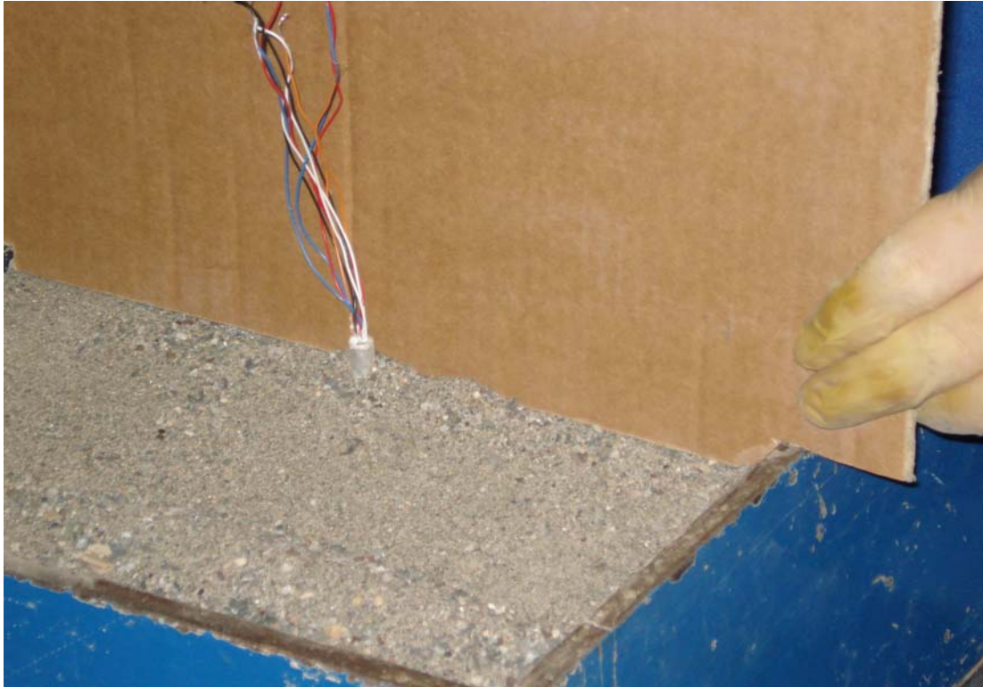
Figure 3.14 Leveling the top of the Shear Box -2-
