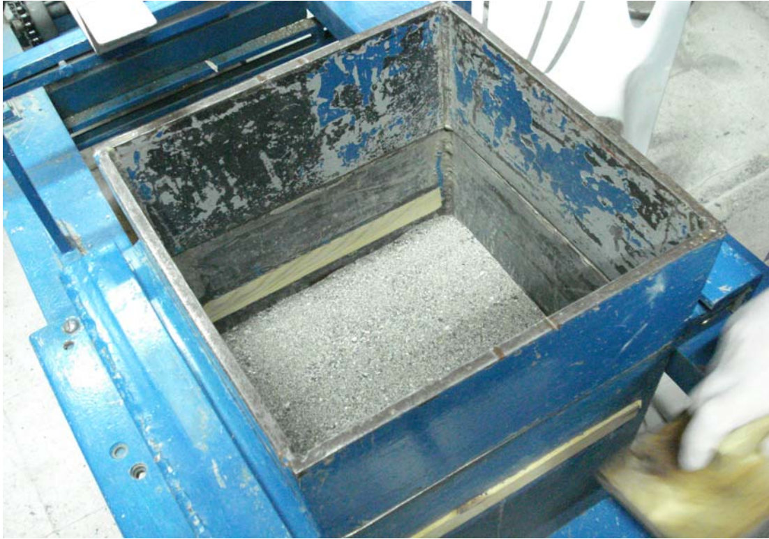
Figure 3.8 Shear Box with Soil before Pile Placement
