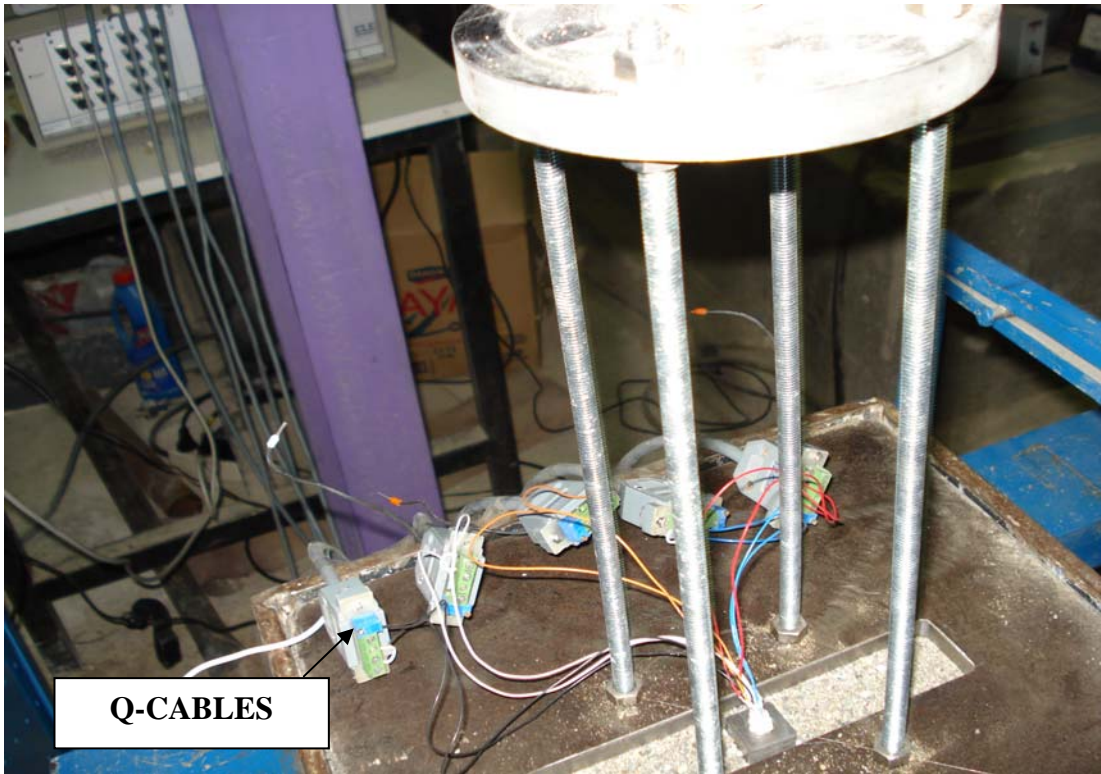
Figure 3.20 Cable Connection in Single Pile Tests
