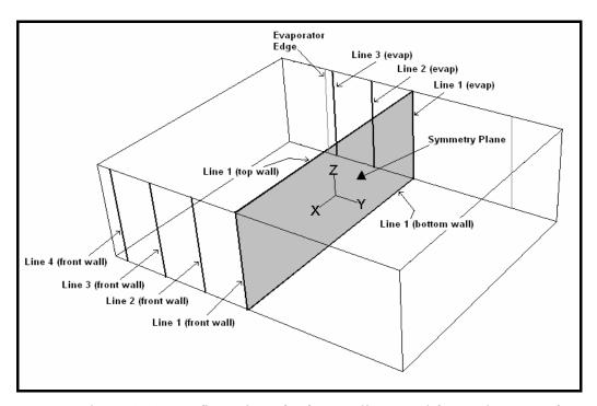
Figure 4.44. Configuration of reference lines used for s.s. heat transfer analysis in the single compartment analysis
