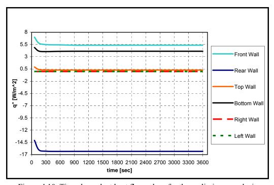
Figure 4.10. Time dependent heat flux values for the preliminary analysis
