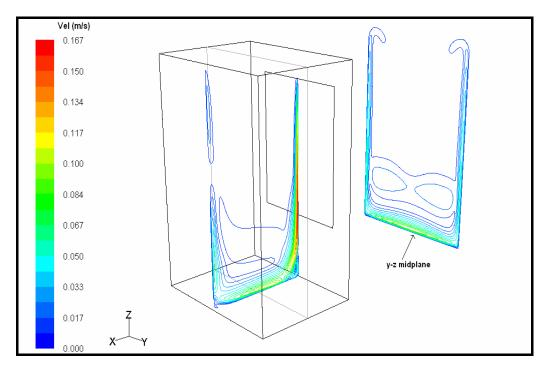
Figure 4.68. Velocity profile for the total refrigerator analysis, t=3600 s (without radiation)
