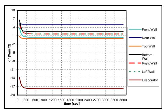
Figure 4.72. Time dependent heat flux values for the total refrigerator analysis (without radiation)
