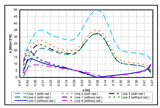
Figure 4.79. Steady state effective heat transfer coefficient values at the front wall for the total refrigerator analysis
