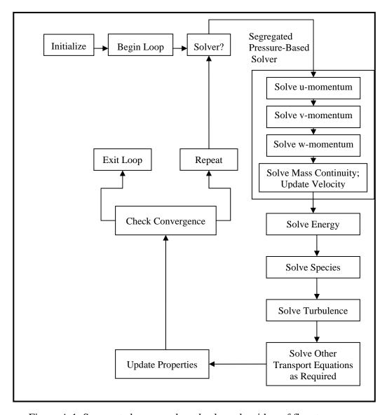
Figure A.1. Segregated pressure based solver algorithm of fluent program
