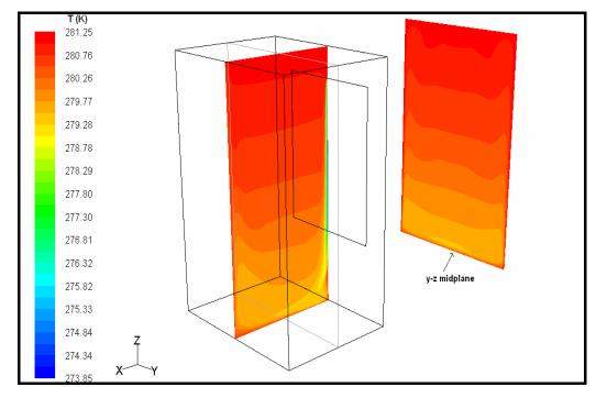
Figure 4.65. Temperature profile for the total refrigerator analysis, t=3600 s (with radiation)
