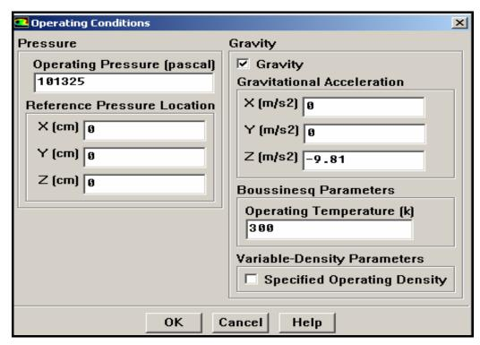
Figure B.5. Operating conditions panel of fluent program
