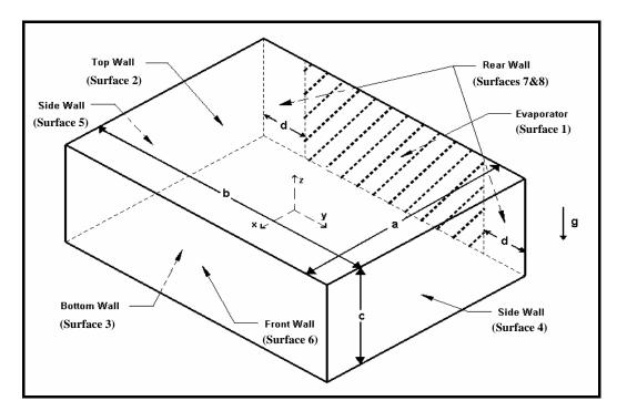
Figure 3.2. Schematic 3-D cavity model of a single compartment for the numerical study based on the experimental work
