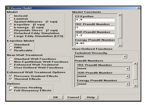
Figure B.2. Viscous model panel of fluent program
