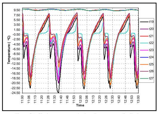
Figure C.1. Single compartment back wall temperature distribution
