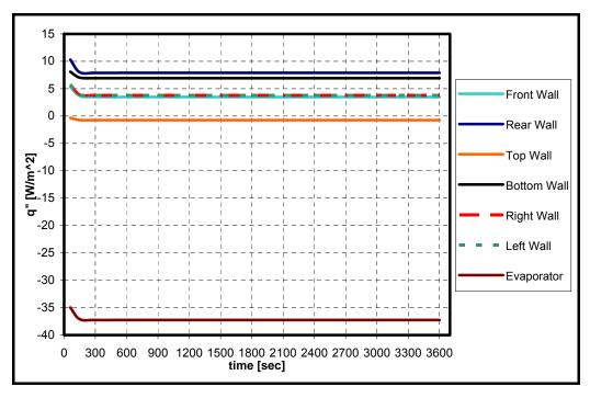
Figure 4.41. Time dependent heat flux values for the single compartment analysis (without radiation)
