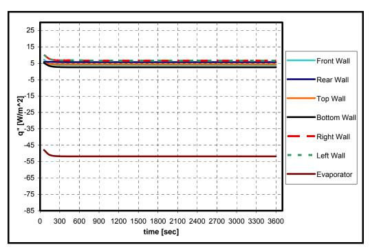
Figure 4.71. Time dependent heat flux values for the total refrigerator analysis (with radiation)
