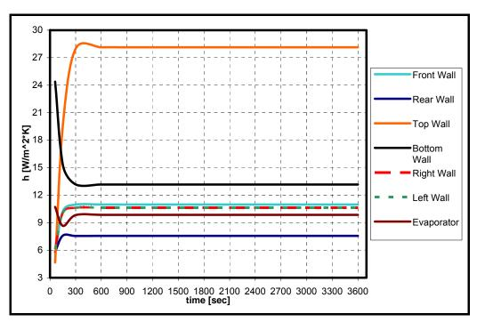
Figure 4.42. Time dependent effective heat transfer coefficient values for the single compartment analysis (with radiation)
