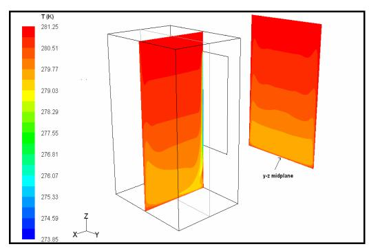
Figure 4.66. Temperature profile for the total refrigerator analysis, t=3600 s (without radiation)
