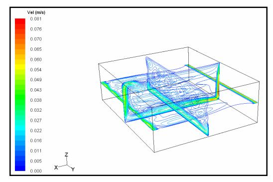
Figure 4.8. Velocity contours at midplanes for the preliminary analysis, t=3600 s
