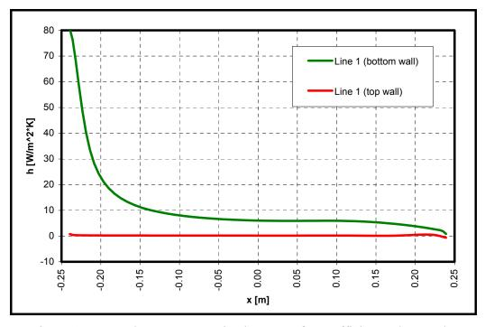
Figure 4.16. Steady state convective heat transfer coefficient values at the bottom and the top walls for the preliminary analysis
