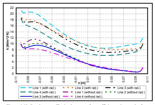
Figure 4.48. Steady state effective heat transfer coefficient values at the front wall for the single compartment analysis
