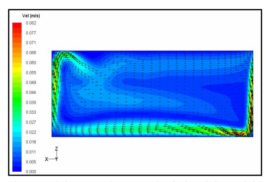
Figure 4.9. Velocity vectors at the symmetry plane for the preliminary analysis, t=3600 s
