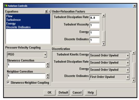
Figure B.7. Continued, Solution controls panel of fluent program
