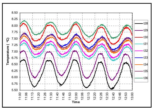
Figure C.2. Single compartment bottom wall temperature distribution
