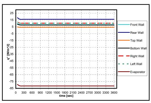
Figure 4.40. Time dependent heat flux values for the single compartment analysis (with radiation)
