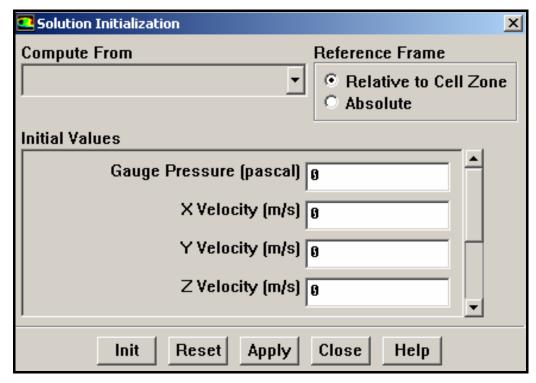
Figure B.9. Solution initialization panel of fluent program
