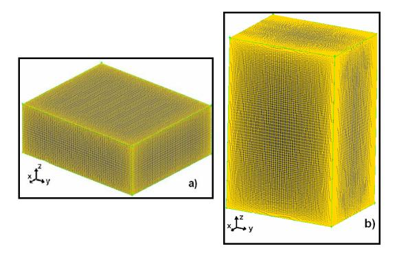
Figure 3.4. Meshed model of 3-D geometries, a) the preliminary study and the single compartment, b) the total refrigerator
