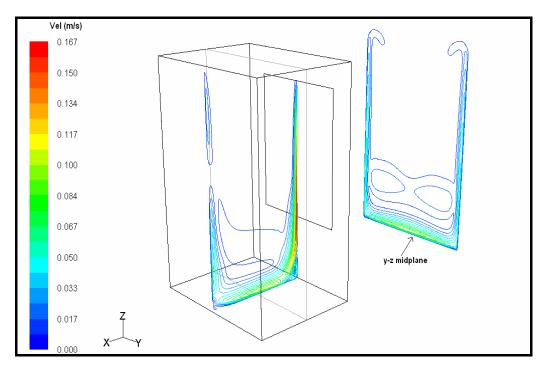
Figure 4.64. Velocity profile for the total refrigerator analysis, t=600 s (without radiation)
