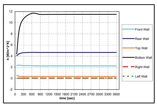
Figure 4.11. Time dependent convective heat transfer coefficient values for the preliminary analysis
