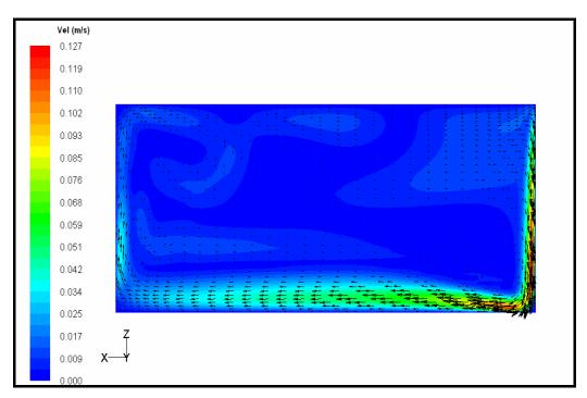
Figure 4.39. Velocity vectors at the symmetry plane for the single compartment analysis, t=3600 s (without radiation)
