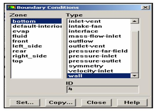
Figure B.6. Boundary conditions panel of fluent program
