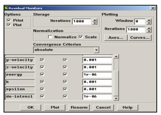
Figure B.8. Continued, Residual monitors panel of fluent program
