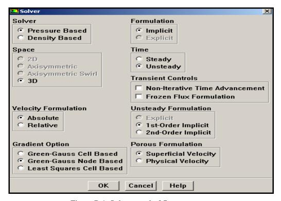
Figure B.1. Solver panel of fluent program
