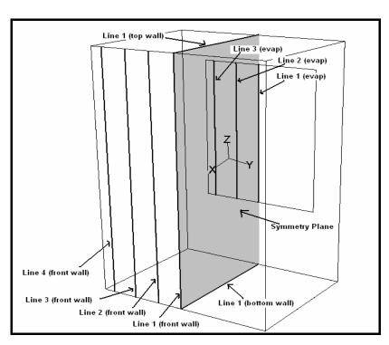
Figure 4.75. Configuration of reference lines used for s.s. heat transfer analysis in the total refrigerator analysis
