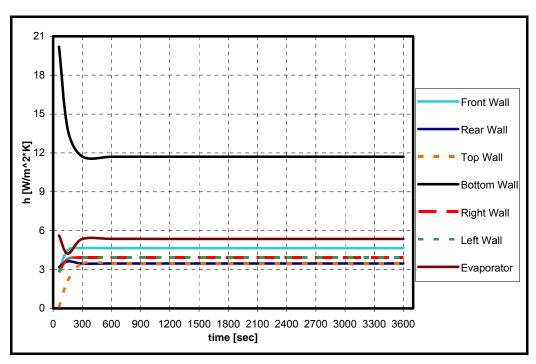
Figure 4.43. Time dependent effective (convective) heat transfer coefficient values for the single compartment analysis (without radiation)
