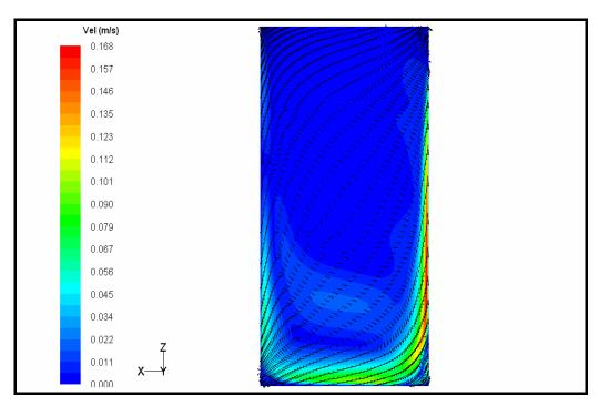
Figure 4.69. Velocity vectors at the symmetry plane for the total refrigerator analysis, t=3600 s (with radiation)
