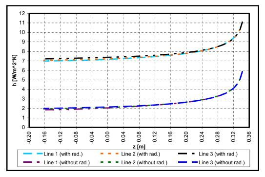
Figure 4.77. Steady state effective heat transfer coefficient values at the evaporator for the total refrigerator analysis
