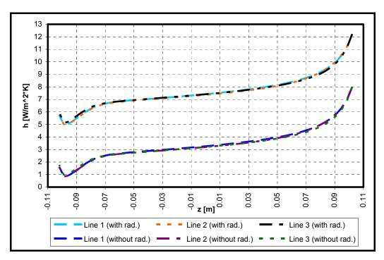
Figure 4.46. Steady state effective heat transfer coefficient values at the evaporator for the single compartment analysis
