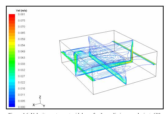
Figure 4.6. Velocity contours at midplanes for the preliminary analysis, t=600 s
