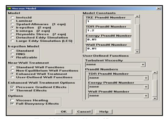
Figure B.2. Viscous model panel of fluent program
