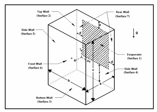
Figure 3.3. Schematic 3-D cavity model of the total refrigerator for the numerical study based on the experimental work
