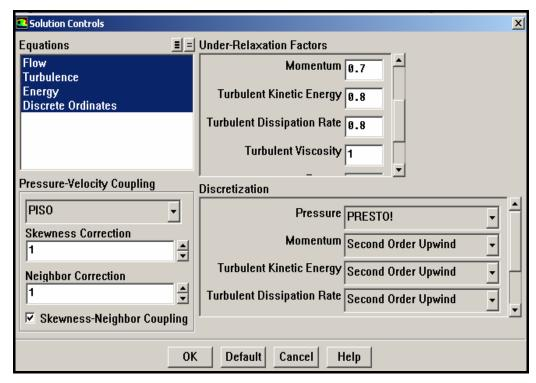
Figure B.7. Solution controls panel of fluent program
