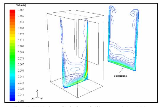
Figure 4.67. Velocity profile for the total refrigerator analysis, t=3600 s (with radiation)
