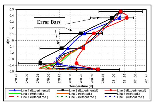
Figure 4.83. Comparison of temperature values on the symmetry plane obtained from the numerical analysis and the experimental work
