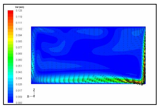
Figure 4.38. Velocity vectors at the symmetry plane for the single compartment analysis, t=3600 s (with radiation)
