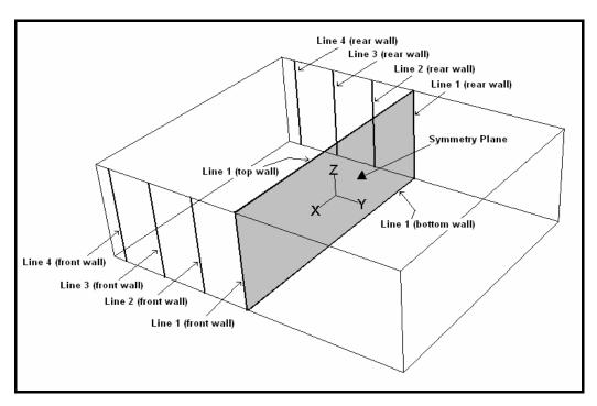
Figure 4.12. Configuration of the reference lines used for s.s. heat transfer analysis in the preliminary analysis
