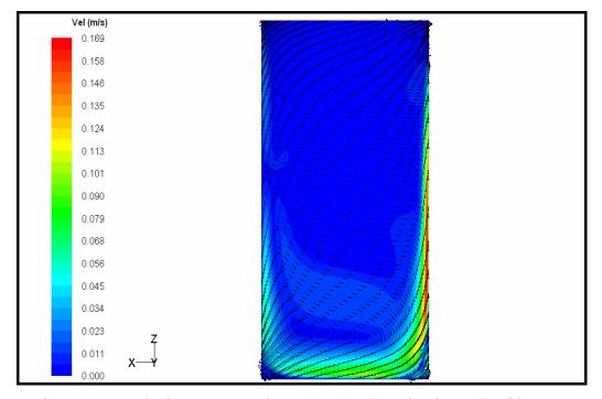
Figure 4.70. Velocity vectors at the symmetry plane for the total refrigerator analysis, t=3600 s (without radiation)
