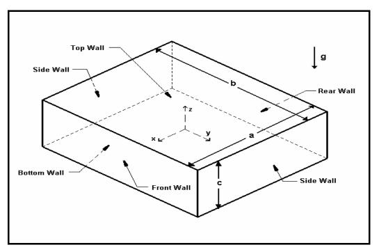
Figure 3.1. Schematic 3-D cavity model for the preliminary study
