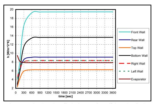
Figure 4.73. Time dependent effective heat transfer coefficient values for the total refrigerator analysis (with radiation)
