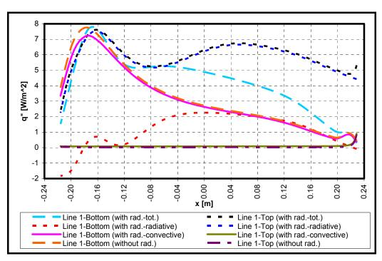
Figure 4.80. Steady state heat flux values at the bottom and the top walls for the total refrigerator analysis
