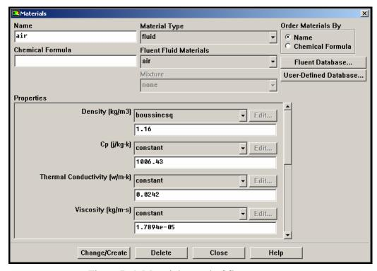
Figure B.4. Materials panel of fluent program
