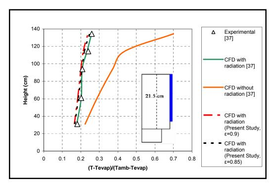
Figure 4.19. Experimental air temperatures and predicted values obtained by the simulation with and without radiation in literature [37] and present study
