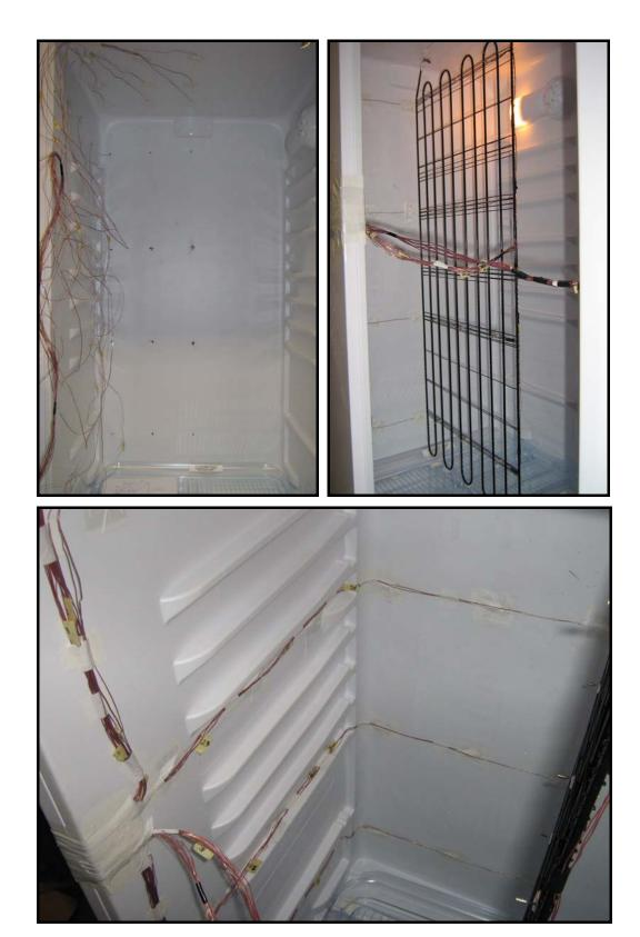
Figure 3.6. Experimental set-up for the total refrigerator
