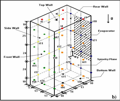
Figure 3.7. Schematic view of the thermocouple locations, a) the single compartment, b) the total refrigerator
