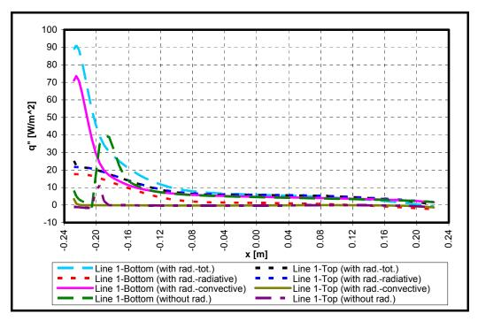
Figure 4.49. Steady state heat flux values at the bottom and the top walls for the single compartment analysis
