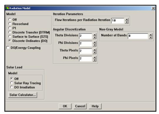
Figure B.3. Radiation model panel of fluent program
