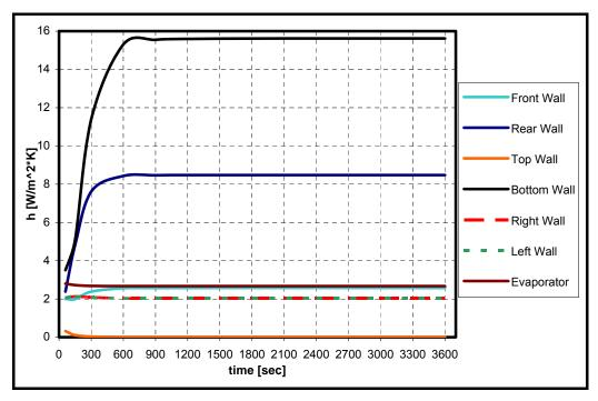
Figure 4.74. Time dependent effective (convective) heat transfer coefficient values for the total refrigerator analysis (without radiation)
