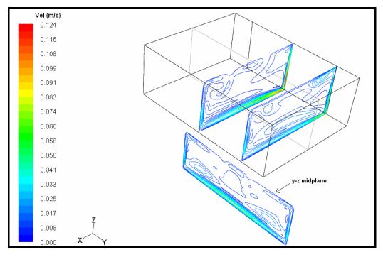
Figure 4.37. Velocity profile for the single compartment analysis, t=3600 s (without radiation)
