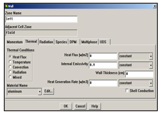
Figure B.6. Continued, Boundary conditions panel of fluent program
