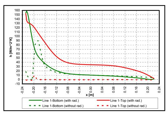
Figure 4.50. Steady state effective heat transfer coefficient values at the bottom and the top walls for the single compartment analysis
