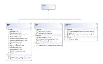
Figure 3.13: SPADE implementation classes in the SPADEX package
