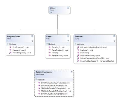
Figure 3.14: Classes in UI Package related with Interface SPADEX coordination
