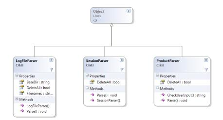
Figure 3.8: Classses in the the Logparser package
