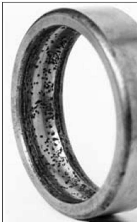
Figure 1.6 Corrosion of the outer ring of a deep groove ball bearing (FAG, 2003)
