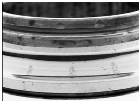
Figure 1.8 False brinelling on a ball bearing (FAG, 2003)
