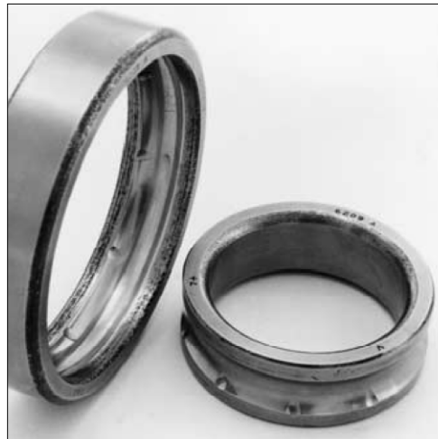
Figure 1.7 Ball indentations in the shoulders of a deep groove ball bearing (FAG, 2003)
