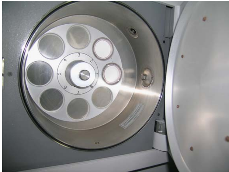
Figure 3.9 The 8-position sample tray
