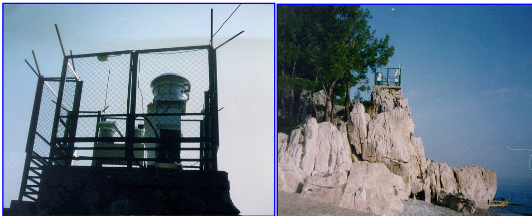
Figure 3.2 The platform onto which Hi-Vol sampler anchored
