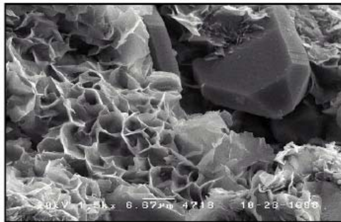
Figure 2.8 SEM Photograph of Montmorillonite (source: http://www.webmineral.com/specimens/Smectite.jpg )
