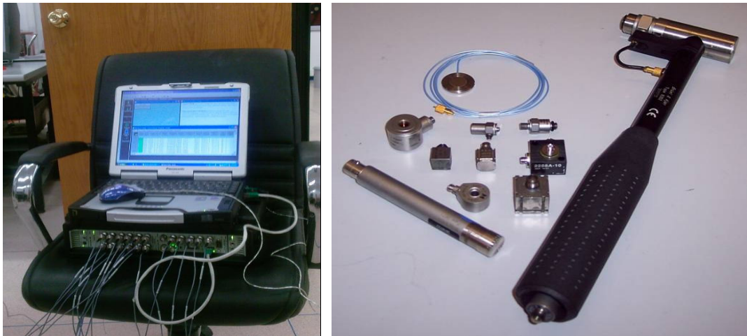
Figure 4.7 View of Data Acquisition System and Modal Hammer
