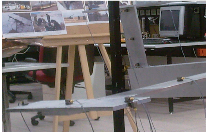
Figure 4.8 View of Measurement Points on the Left Wing and Vertical Stabilizer
