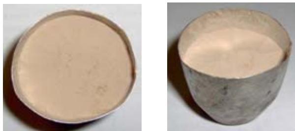
Figure 3.3: Raw meal in platinum crucible
