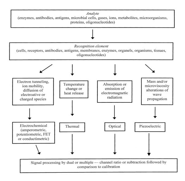
Figure 1.2. Biocomponent and transducers employed in construction of biosensors (Mello & Kubota, 2002)
