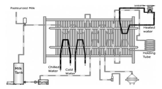
Figure 1.3 The representative figure of pasteurizer of milk (Riverol et al., 2008)
