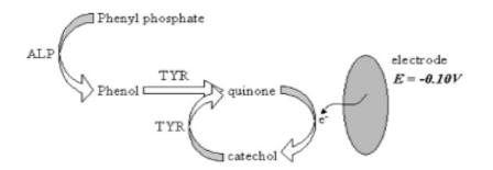
Figure 1.4.Schematic representation of alkaline phosphatase detection at the graphite–Teflon–tyrosinase electrode (Serra et al., 2005)
