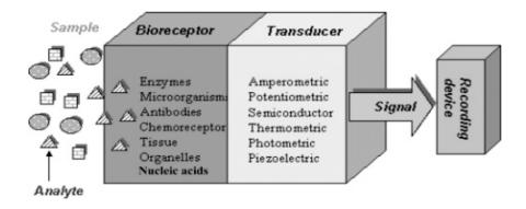
Figure 1.1.The representative figure of biosensor and its components (Newman *et al.* 2004; Terry *et al.*, 2005)
