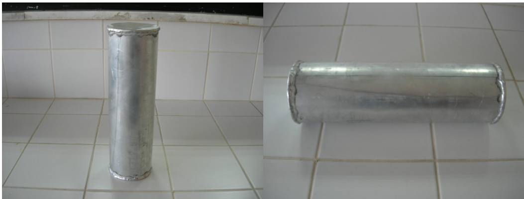
Figure 3.14 The extrusion billets composed of compacts.
