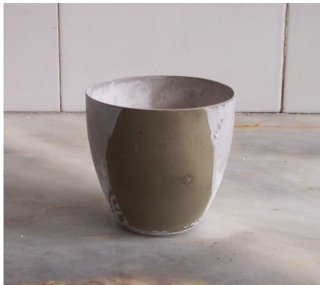
Figure 3.2 Nickel crucible used for calcination.
