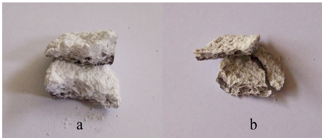
Figure 4.22 Products obtained from experiments as they come out of the furnace. a) 0.25 g h-BN + 1 g CaO + 3 g B 2 O 3 mixture, experiment conducted under Nitrogen gas, b) 0.25 g h-BN + 1 g CaO + 3 g B 2 O 3 mixture, experiment conducted under Argon gas.
