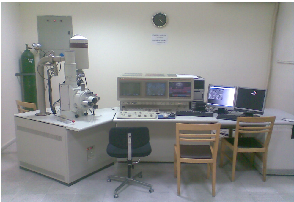
Figure 3.6 JSM – 6400 scanning electron microscope.
