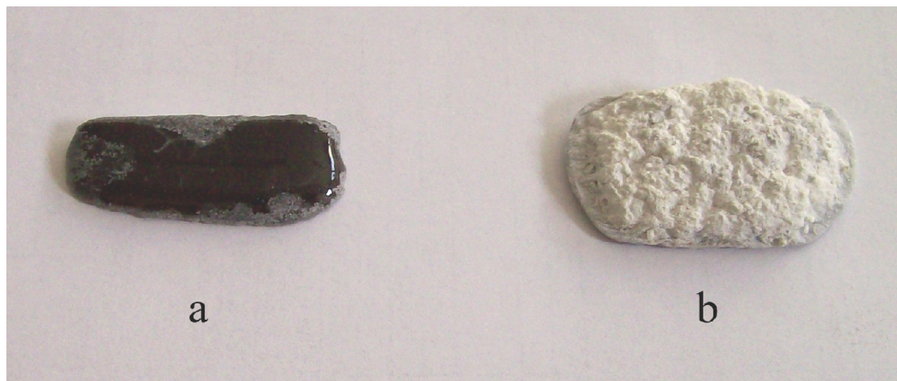
Figure 4.21 Samples as they come out of the furnace. a) C free 25 wt.% CaO – B 2 O 3 mixture, b) C free 25 wt.% CaO – B 2 O 3 and h-BN addition for nucleation.
