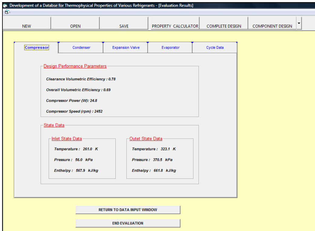
Figure 9.5 Example cycle design output parameters for compressor
