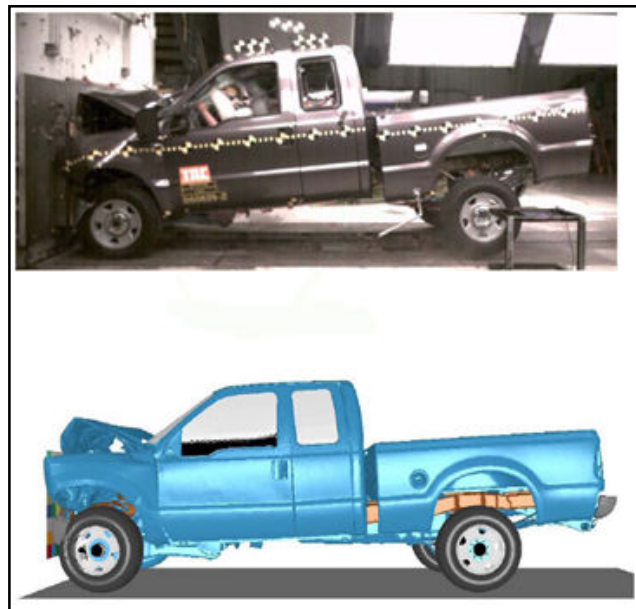
Figure 2.4 Validation of finite element model of Ford F250 with test [25]
