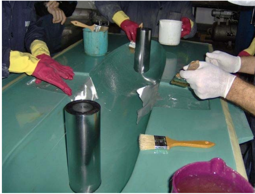
Figure 6.4 Hand lay-up process for the vehicle body
