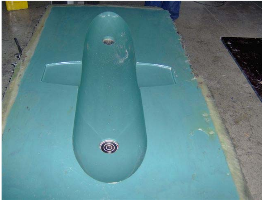
Figure 6.3 Mold of the vehicle (finished product)
