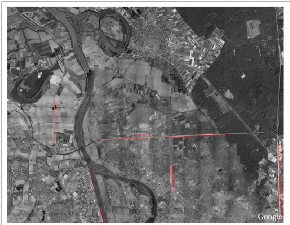
Figure A.25: ETOR – Final result (overlaid on original image). Instead of the runway a series of long straight road segments are detected.
