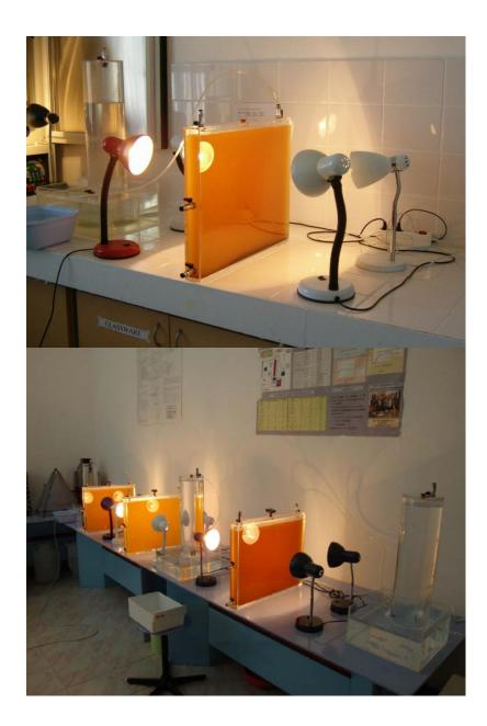
Figure 3.2 The indoor hydrogen production experimental setup using *R. capsulatus* YO3 (Hup<sup>-</sup>).
