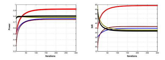
**Figure** 4.6: Evolutions of Power and SIR in synchronous update algorithm of Eq. (4.7) with  $P_{min} = 0.3$  and  $\Delta = 0.01$ .
