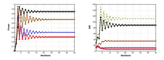
**Figure** 4.4: Evolutions of power and SIR are illustrated for  $P_{min} = 0.3$ . Users have perfect knowledge of congestion level at their intended receiver and synchronously react by changing their power levels.
