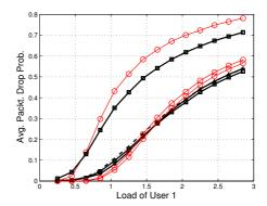
Figure 5.10: The performance of buffer partitioning under MMPA with modulating Markov chain transition probabilities equal to 0.5. Arrival rate is  $0.2\lambda$  and  $1.8\lambda$  according to the state of the Markov chain.
