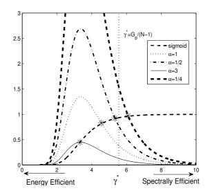
Figure 2.5:  $\gamma^*$  is the intersection of two functions  $f(\gamma)$  and  $\frac{1}{\alpha}f'(\gamma)\gamma$ . The horizontal axis component of intersection points is the equilibrium SINR  $\gamma^*$ . For  $\alpha < 1$ , as the priority of spectral efficiency is higher,  $\gamma^*$  takes higher values. It is not possible for users to mutually reach  $\gamma^*$  in case  $\gamma^* > \frac{G_p}{K-1}$
