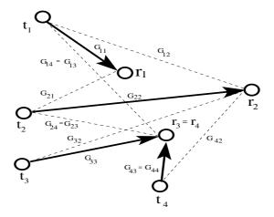
Figure 4.1: The ad-hoc wireless network model: A set of interfering links
