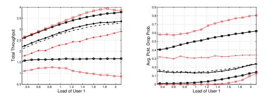
**Figure** 5.9: N=5 and B=5 buffer per user. A realistic unbalanced load regime: x-axis represents load of user 1 and  $\rho_2 = 0.2$   $\rho_3 = 0.8$ ,  $\rho_4 = 0.3$ ,  $\rho_5 = 0.9$
