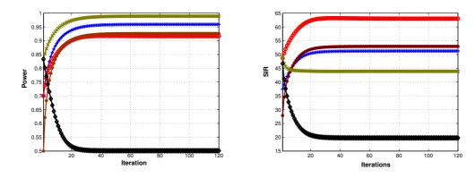
**Figure** 4.5: Evolutions of Power and SIR in synchronous update algorithm of Eq. (4.7) with  $P_{min} = 0.5$  and  $\Delta = 0.05$ .
