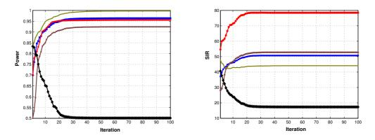
Figure 4.7: Evolutions of Power and SIR in synchronous update algorithm of Eq. (4.12) with erroneous feedback information.  $P_{min} = 0.5$ ,  $\xi = 0.5$  and  $\Delta = 0.05$ .
