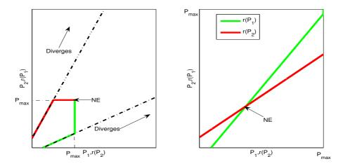
Figure 3.2: Illustration of reaction curves of two players for feasible and infeasible cases. On the left,  $\lambda_{PF} > \frac{1}{SIR^{obj}}$ , for the selected gain values, hence the feasible set is empty. NE is shown for  $P_{max} = 1$ . For  $P_{max} \to \infty$ , power of users diverge. On the right,  $\lambda_{PF} < \frac{1}{SIR^{obj}}$
