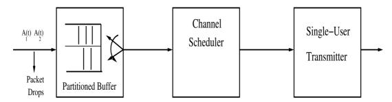
Figure 5.4: The model for two user joint buffer management and user scheduling in a time-varying channel
