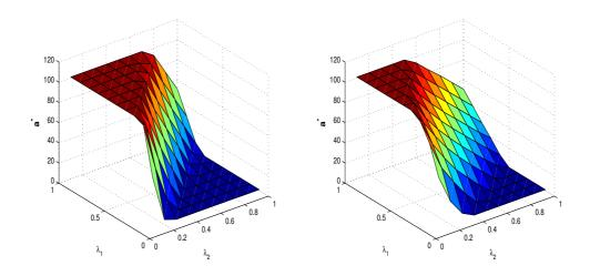
Figure 5.5: The joint optimal scheduling probability  $a^*$  in (%) is plotted with respect to  $(\lambda_1, \lambda_2)$  plane. B = 20 buffers per user.  $P_0 = 0.6$  and  $P_0 = 0.4$  on the left and right plots respectively.
