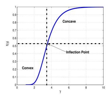
Figure 2.2: Function  $f(\gamma)$  v.s.  $\gamma$  in normal scale. It is plotted for BPSK modulation with packet length L=400 bits.
