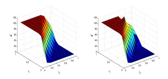
Figure 5.6: The joint optimal scheduling probability  $a^*$  in (%) is plotted with respect to  $(\lambda_1, \lambda_2)$  plane.  $P_0 = 20$ . B = 20 and B = 5 on the left and right plots respectively.
