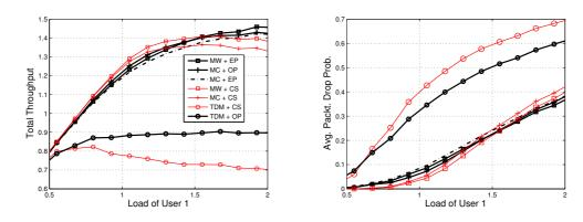
Figure 5.7: N=2 and B=5 buffers per user. x-axis represents load of user 1.  $\rho_2 = 0.3$
