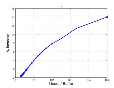
Figure 5.2: The percentage increase in total throughput v.s. users per buffer. Optimal buffer allocation is compared to even buffer allocation in parallel  $M/M/1/m_i$  system with a total buffer of B=3500. There are two classes of users. 25% of users belong to first class and the remaining belongs to the second.  $\rho_1=11\rho_2=1.1$ . As more users share the buffers, buffer allocation yields higher increase in throughput.
