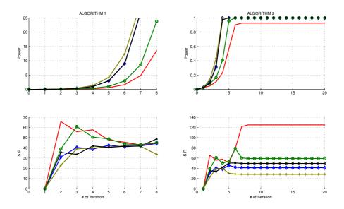
**Figure** 3.5: Evolutions of power and SIR for algorithms 1 and 2. Note that algorithm 1 in (3.1) diverges in just a few iterations. Algorithm 2 has an equilibrium due to finite power limit. Yet, it is inefficient as users transmit with powers nearly equal to  $P_{max}$
