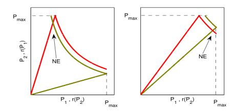
Figure 3.4: Possible reaction curves for different channel gains in a two transmitter-receiver system. Linear portion of reaction curves represent the set of power allocations in which the user attains the SIR objective. Note that the objectives are infeasible for both cases.
