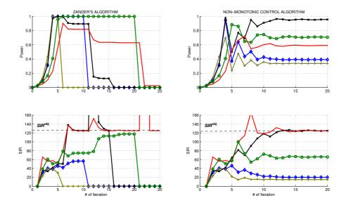
**Figure** 3.6: Evolutions of power and SIR values for Algorithm 3 and NMPC. Algorithm 3 removes users 2,1,3 and 5 respectively so that the objective is feasible. In NMPC, users 3 and 4 reach the objective while the others operate in a lower outage. Zig-zags are due to non-monotonic reaction curves of users.
