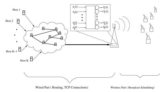
**Figure** 5.1: A network with a wireless last mile: Multiple sessions sharing a finite buffer space are taking scheduled service in a wireless downlink.
