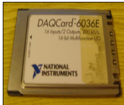
Figure 4.26 A view of data acquisition card
