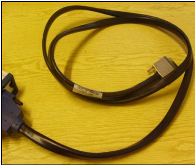
Figure 4.25 A view of data acquisition cable
