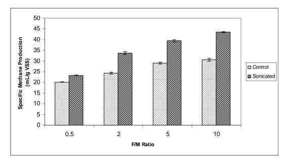
Figure 4.29. Methane gas amount of 250 mL reactors at different F/M ratios as per gram VSS after anaerobic digestion
