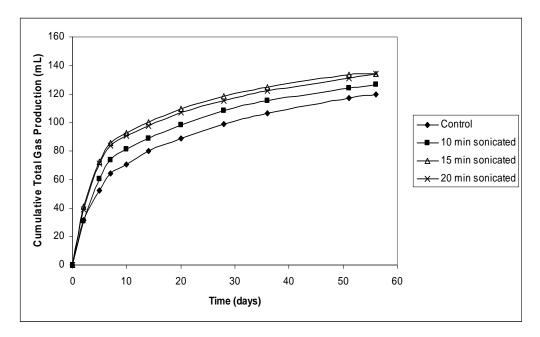
Figure 4.24. Cumulative total gas production of sludges sonicated at different times during anaerobic digestion
