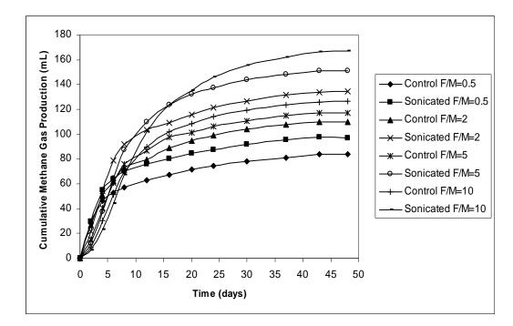
Figure 4.33. The daily change in cumulative methane gas production of 250 mL reactors at different F/M ratios during anaerobic digestion
