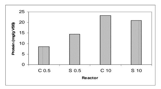
Figure 4.44. Protein content of 3 L reactors at different F/M ratios after digestion
