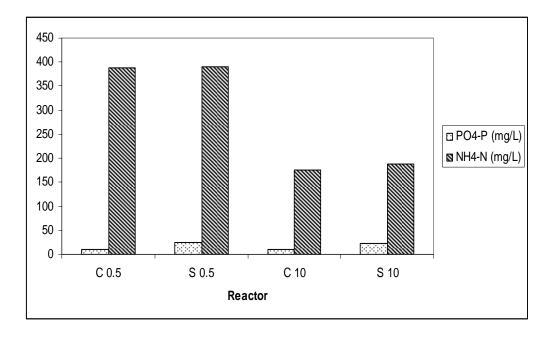
Figure 4.45. Phosphorus and nitrogen content of 3 L reactors at different F/M ratios after digestion
