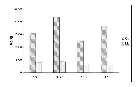
Figure 4.47. Calcium and magnesium concentration in 3 L reactors at different F/M ratios after digestion
