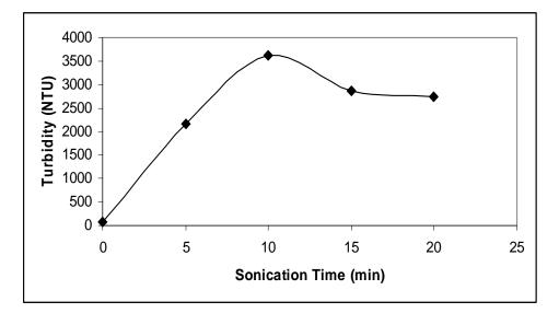
Figure 4.10. The variation in turbidity according to sonication time (using 14 mm probe)
