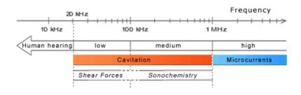
Figure 2.2. The sonication frequency interval (Ultrawaves, 2008)
