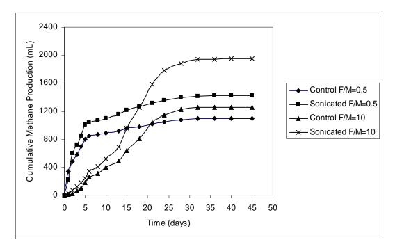
Figure 4.39. The daily change in cumulative methane gas production of 3 L reactors at different F/M ratios during anaerobic digestion
