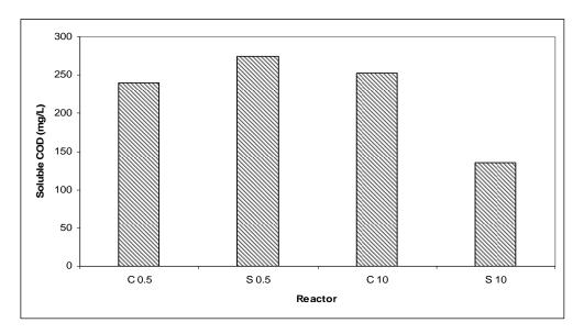
Figure 4.41. Soluble COD of 3 L reactors at different F/M ratios after digestion
