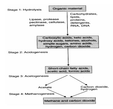
Figure 2.1. Schematic Representation of Anaerobic Digestion (Scragg, 2005)
