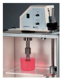
Figure 3.1. Ultrasonic homogenizer
