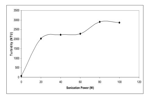
Figure 4.7. The variation in turbidity according to sonication power (using 14 mm probe)
