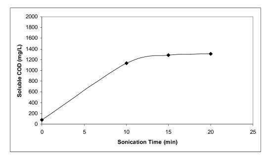
Figure 4.23. Soluble COD concentration in sludges sonicated at different times before digestion
