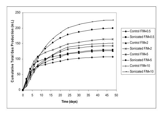
Figure 4.32. The daily change in cumulative total gas production of 250 mL reactors at different F/M ratios during anaerobic digestion
