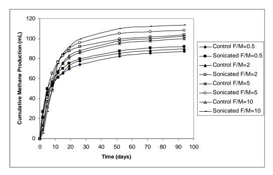
Figure 4.27. The daily change in cumulative methane gas production of 250 mL reactors at different F/M ratios during anaerobic digestion
