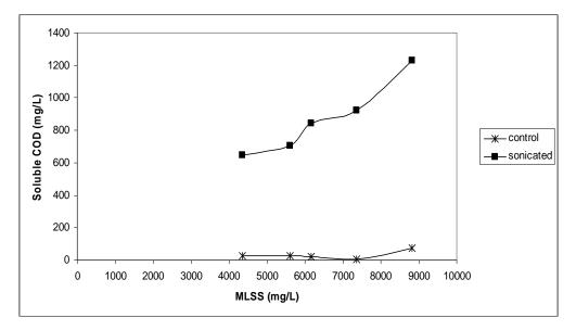
Figure 4.12. Change in soluble COD with respect to MLSS concentration of sludge
