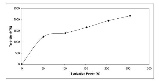
Figure 4.18. The variation in turbidity according to sonication power (using 22 mm probe)
