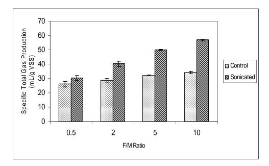
Figure 4.34. Total gas amount of 250 mL reactors at different F/M ratios as per gram VSS after anaerobic digestion
