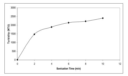
Figure 4.21. The variation in turbidity according to sonication time (using 22 mm probe)
