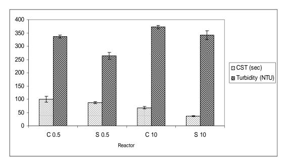
Figure 4.40. CST and turbidity values of 3 L reactors at different F/M ratios after digestion
