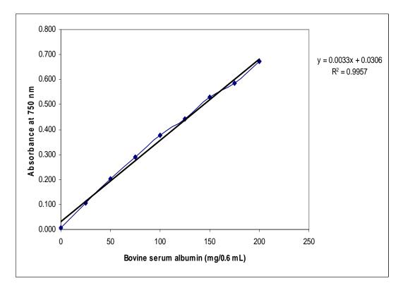
Figure A.2. The calibration curve obtained for the protein analysis
