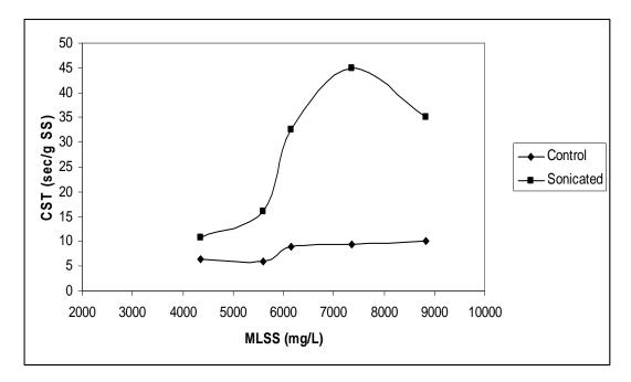
Figure 4.14. Change in CST with respect to MLSS concentration of sludge
