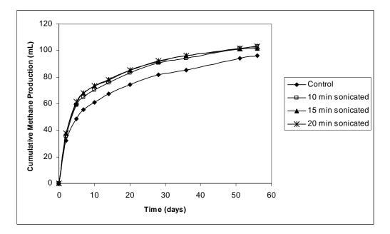
Figure 4.25. Cumulative methane gas production of sludges sonicated at different times during anaerobic digestion
