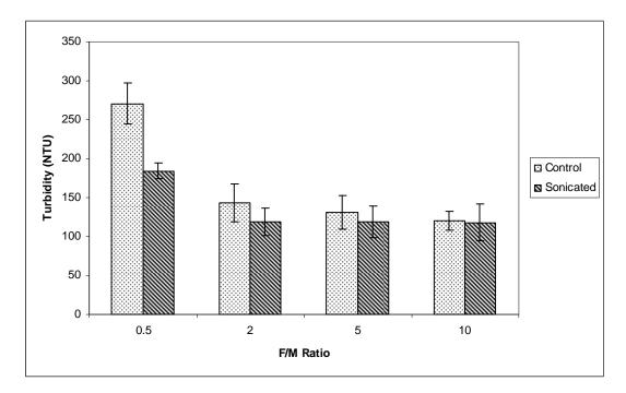
Figure 4.31. Turbidity values of 250 mL reactors at different F/M ratios after digestion
