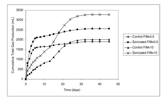
Figure 4.38. The daily change in cumulative total gas production of 3 L reactors at different F/M ratios during anaerobic digestion
