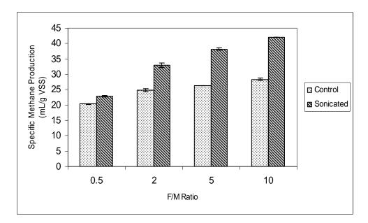
Figure 4.35. Methane gas amount of 250 mL reactors at different F/M ratios as per gram VSS after anaerobic digestion
