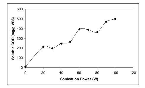
Figure 4.1. The variation in soluble COD according to sonication power (without temperature control)
