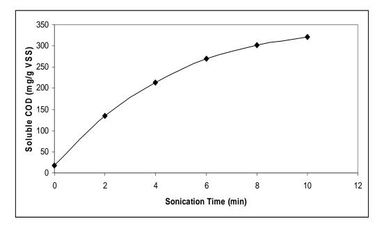
Figure 4.19. The variation in soluble COD according to sonication time (using 22 mm probe)
