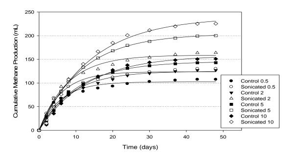
Figure C.2. Representation of non-linear regression analysis of methane gas productions of 250 mL unsonicated and high power-sonicated reactors
