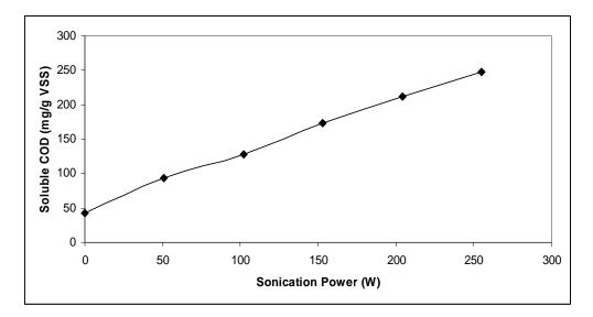
Figure 4.16. The variation in soluble COD according to sonication power (using 22 mm probe)
