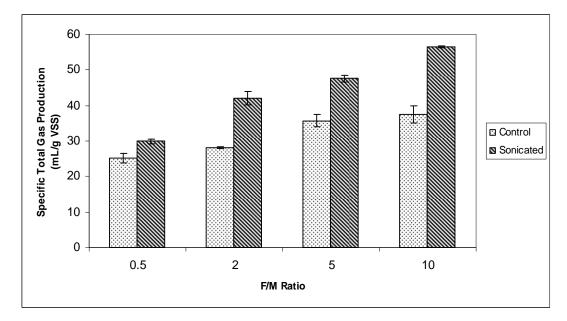
Figure 4.28. Total gas amount of 250 mL reactors at different F/M ratios as per gram VSS after anaerobic digestion
