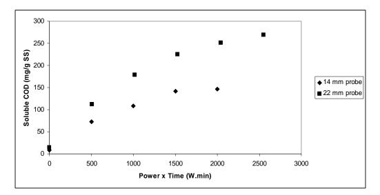
Figure 4.22. The comparison of probes as soluble COD according to sonication power x time
