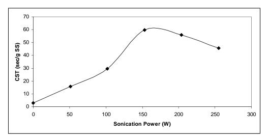
Figure 4.17. The variation in CST according to sonication power (using 22 mm probe)
