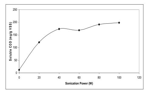
Figure 4.5. The variation in soluble COD according to sonication power (using 14 mm probe)
