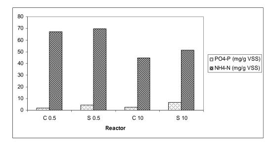
Figure 4.46. Normalized phosphorus and nitrogen content of 3 L reactors at different F/M ratios after digestion
