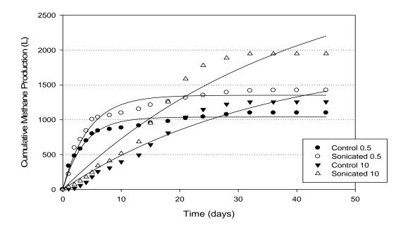
Figure C.3. Representation of non-linear regression analysis of methane gas productions of 3 L unsonicated and high power-sonicated reactors
