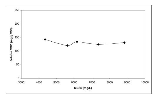
Figure 4.13. Change in normalized soluble COD with respect to MLSS concentration of sludge
