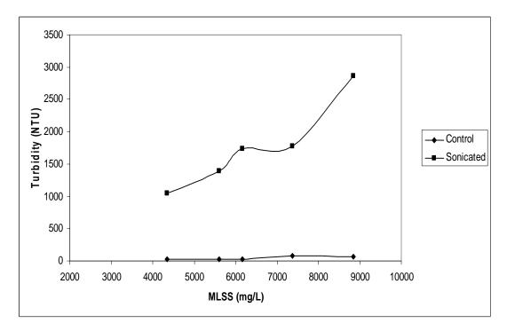
Figure 4.15. Change in turbidity with respect to MLSS concentration of sludge
