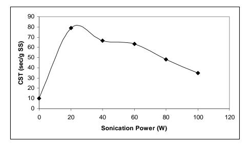
Figure 4.6. The variation in CST according to sonication power (using 14 mm probe)
