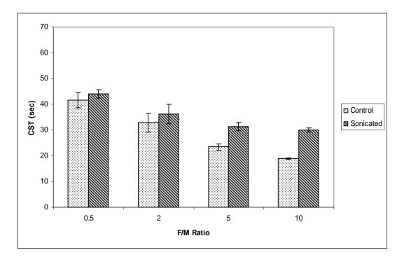
Figure 4.30. CST values of 250 mL reactors at different F/M ratios after digestion
