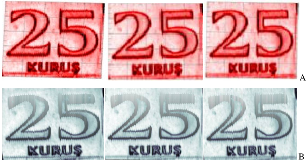
Figure 3.10 Images of the same part of 25 Turkish Kuruş for different z axis. First image was taken when z axis is on 52000 counts, middle image was taken on focus point which is 72000 counts and the last image was taken when z axis is on 72000 counts (A), matlab graphs of the same images (B)
