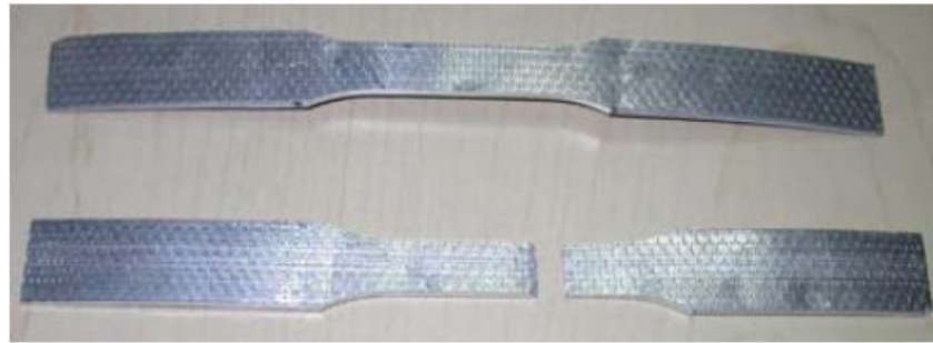
Figure 4.5 Solutionized aluminum tensile test specimen deformed through patterned portion of the roll.
