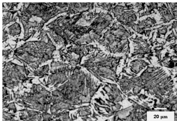
Figure 5.9 Optical micrograph of the undeformed sample (Etched in 2% Nital solution for 15 seconds and in Picral solution for 30 seconds)
