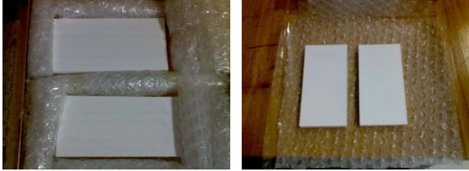
Figure 5.15 hBN target plates produced in Eskişehir Anadolu University
