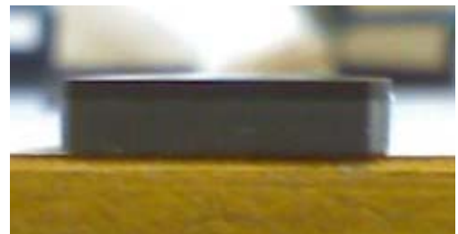
Figure VIII.1. TNMN-323T, PcBN turning insert- top and side views
