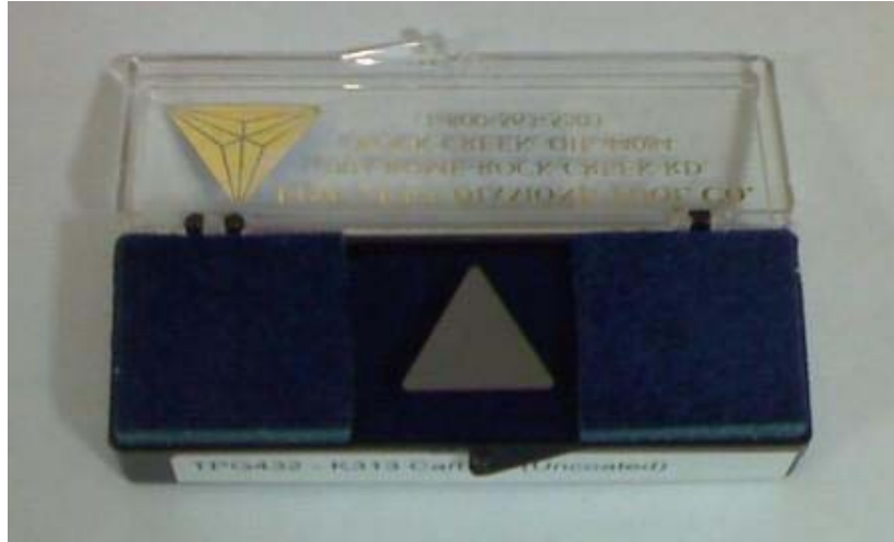
Figure VIII.3. TPG432, uncoated Tungsten Carbide turning insert- top view
