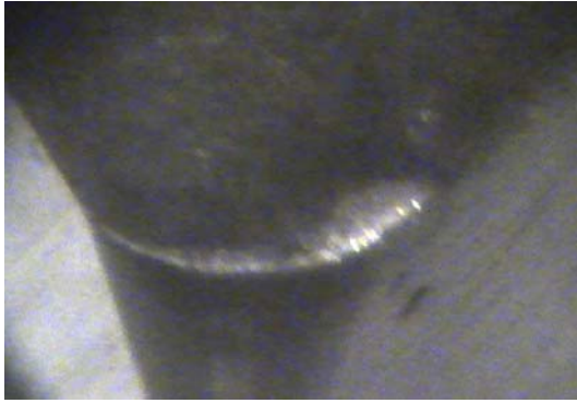
Uncoated WC V=50 m/min, a_p=2 mm, f=0.1 mm
