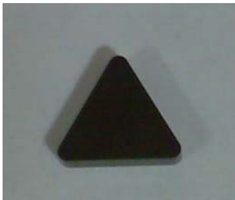
Figure VIII.1. TNMN-323T, PcBN turning insert- top and side views
