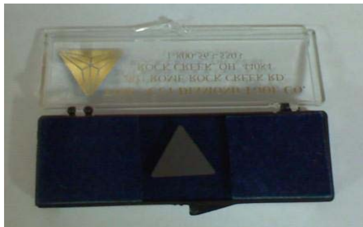
Figure VIII.4. TiAlN coated Tungsten Carbide turning insert-top view
