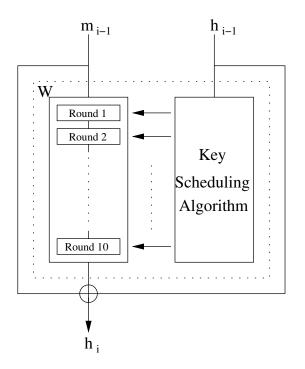
Figure 4.21: Compression Function of Whirlpool Hash Function
