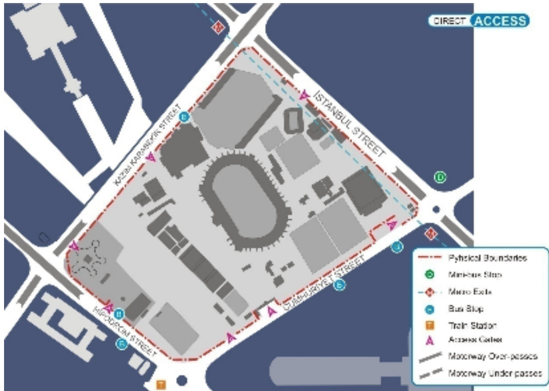
Fig. 4.11 Under and over passes, bus stops, and metro connections providing vehicular access on the edges of the site.
