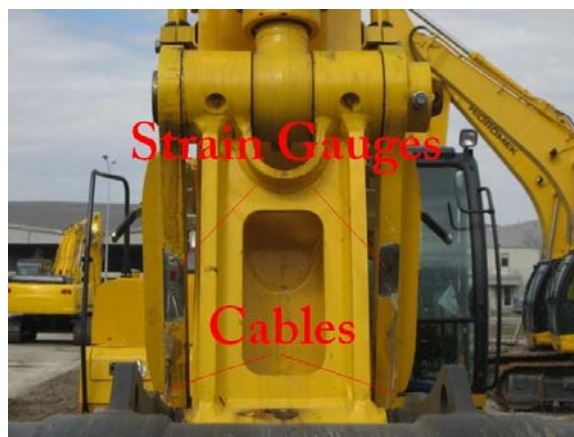
Figure 4.14 – Strain Gauges and Cables
