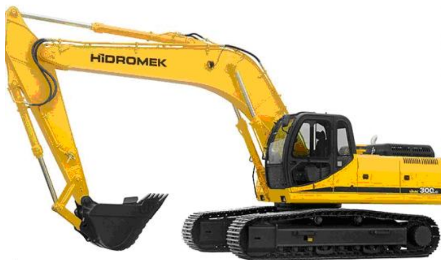
Figure 1.2 - A typical crawler type excavator
