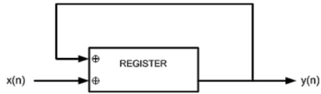
Figure 13: Addition block of Sinc filter.
