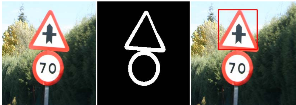
Figure 4.2 Sample misdetection of a circular sign for a merged sign
