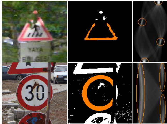
Figure 3.15 Two samples of traffic signs with bad visual conditions, their segmented major components and their line histograms
