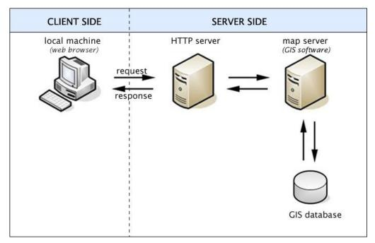
Figure 2.1 A typical approach for client-server architecture
