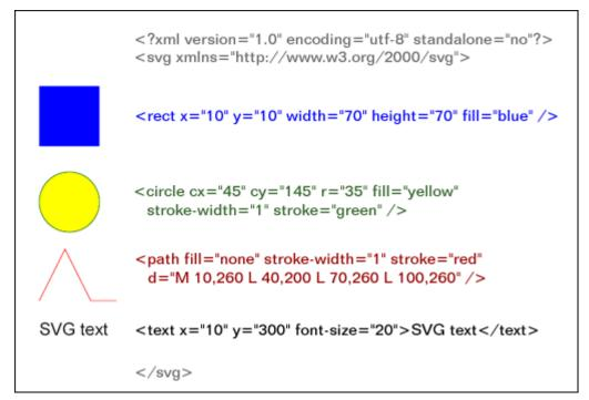
Figure 3.2 SVG source code of simple graphical objects
