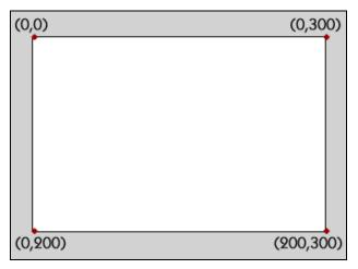
Figure 4.4 Initial coordinate system of a SVG viewport
