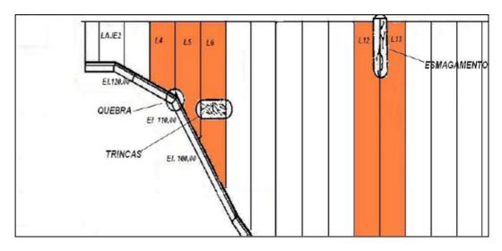
Figure 3.11 Face slab cracks of Xingó Dam (Souza, 2007)
