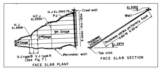
Figure 3.6 Face slab layout of Golillas Dam (Marulanda and Amaya, 1985)
