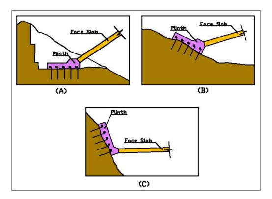
Figure 2.5 Different plinth types (Mori and Mataron, 2000) (A) Horizontal plinth, (B) Sloping plinth, (C) Vertical plinth
