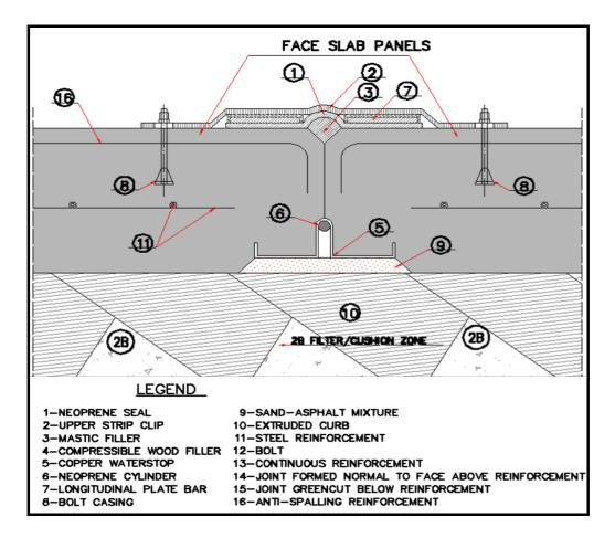
Figure 4.10 Details of vertical expansion joints of Gökçeler Dam (Hidro Dizayn, 2007-c)
