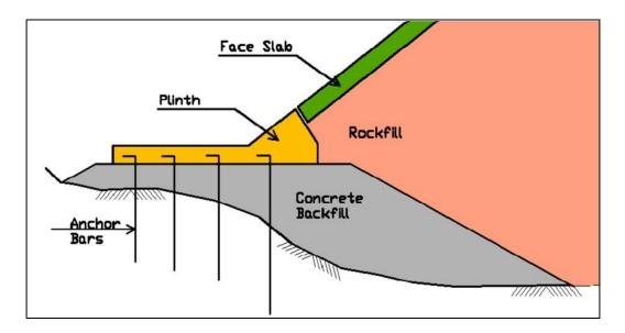
Figure 2.7 Typical cross-section of thick plinth (Kleiner, 2005-d)
