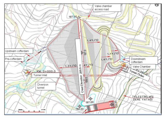
Figure 4.7 General layout of CFRD formulation (Hidro Dizayn, 2007-b)
