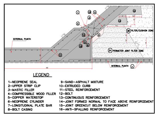
Figure 4.9 Horizontal plinth cross-section of Gökçeler Dam (Hidro Dizayn, 2007-c)
