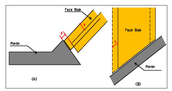
Figure 2.11 Perimeter joint movements (Hedien, 2005-a)
