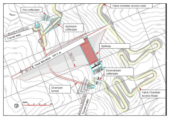
Figure C.1 General layout of RCC formulation (Hidro Dizayn, 2007-b)
