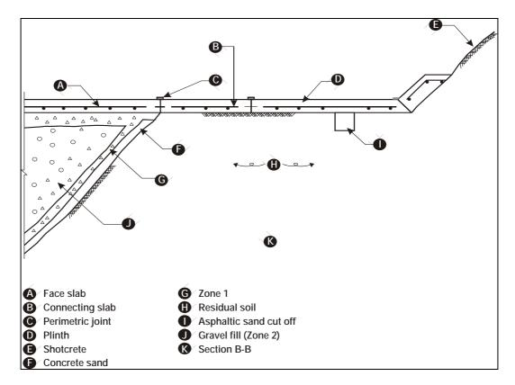
Figure 3.7 Salvajina Dam plinth founded on residual soil (Kleiner, 2005-e).
