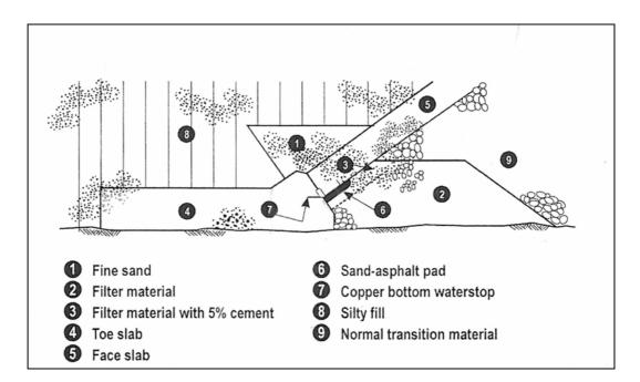
Figure 2.13 Upper barrier of cohesionless fine deposit (Hedien, 2005-a)
