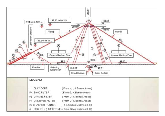
Figure B.2 Main cross-section ECRD type (Hidro Dizayn, 2007-b)
