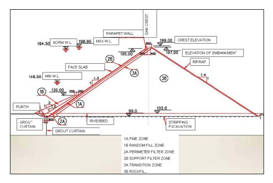
Figure 4.8 Main cross-section of CFRD type (Hidro Dizayn, 2007-b)
