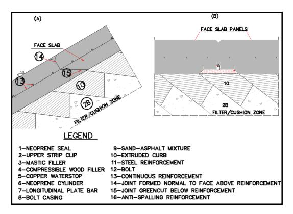
Figure 4.11 Horizontal construction and vertical contraction joints (Hidro Dizayn, 2007-c)
