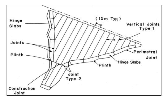
Figure 3.5 Face slab layout of Alto Anchicaya Dam (Materon, 1985).
