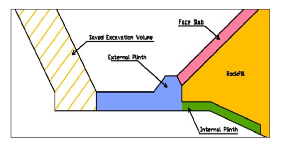
Figure 2.8 Internal and external plinth combination (Kleiner, 2005-d)
