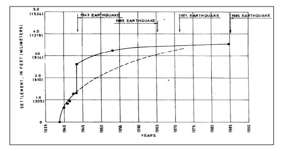
Figure 3.3 Crest settlement curve for Cogoti Dam (Arrau et al., 1985).
