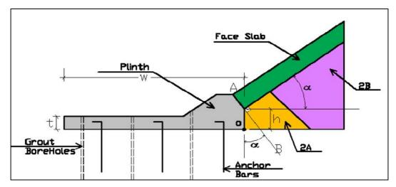
Figure 2.6 Basic geometry of conventional plinth (Cooke, 2000-b).
