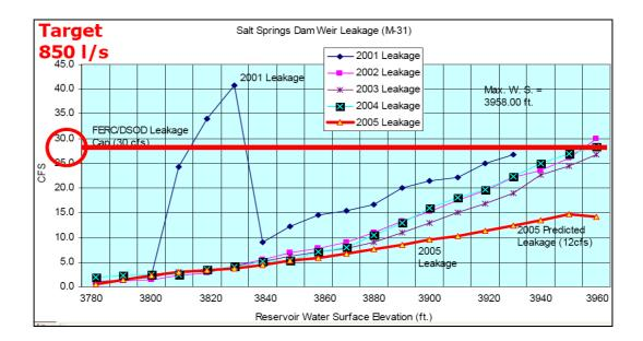
Figure 3.2 Leakage rates of Salt Springs Dam against reservoir head (Scuero, 2007)
