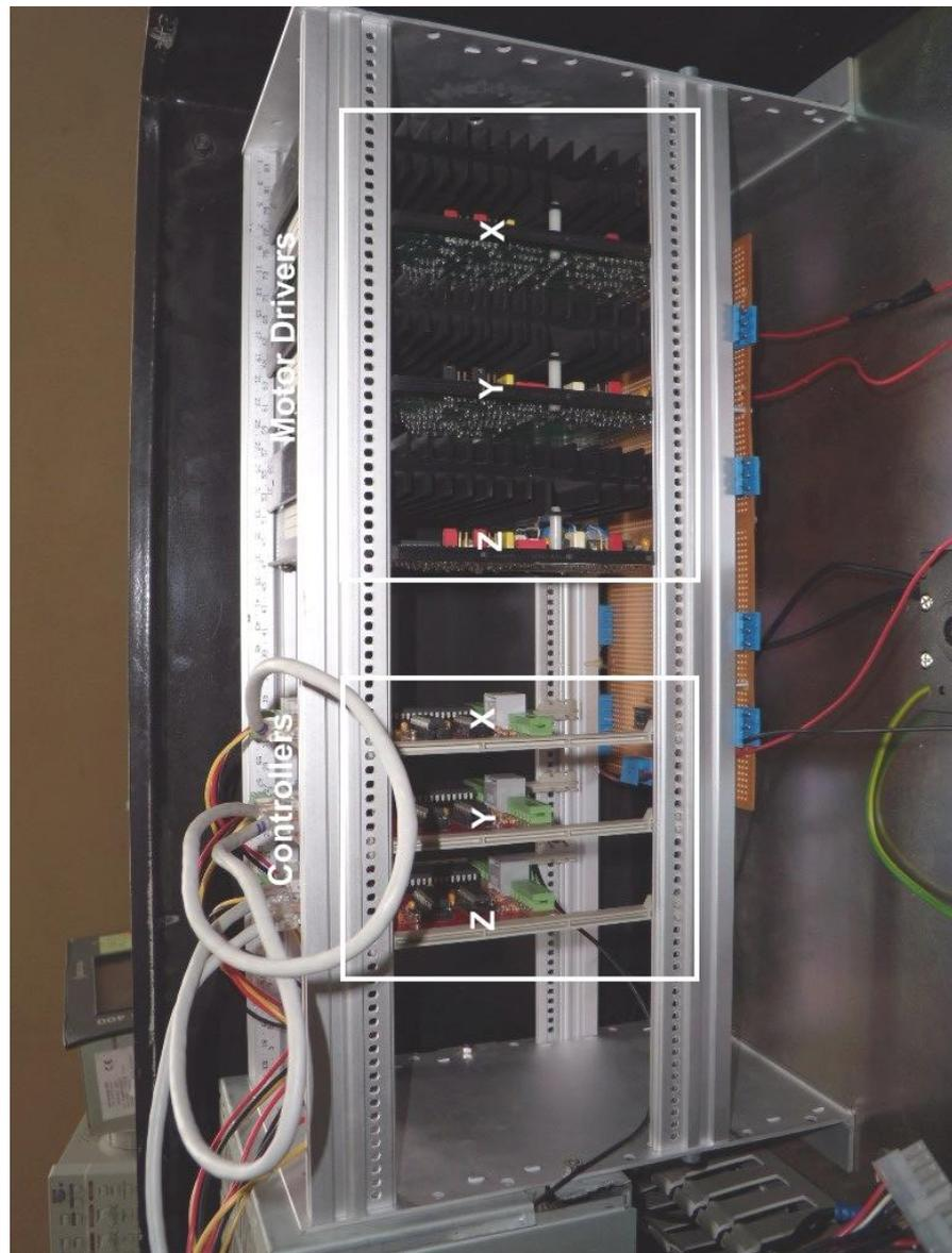
**Figure 5.6** Developed control system
