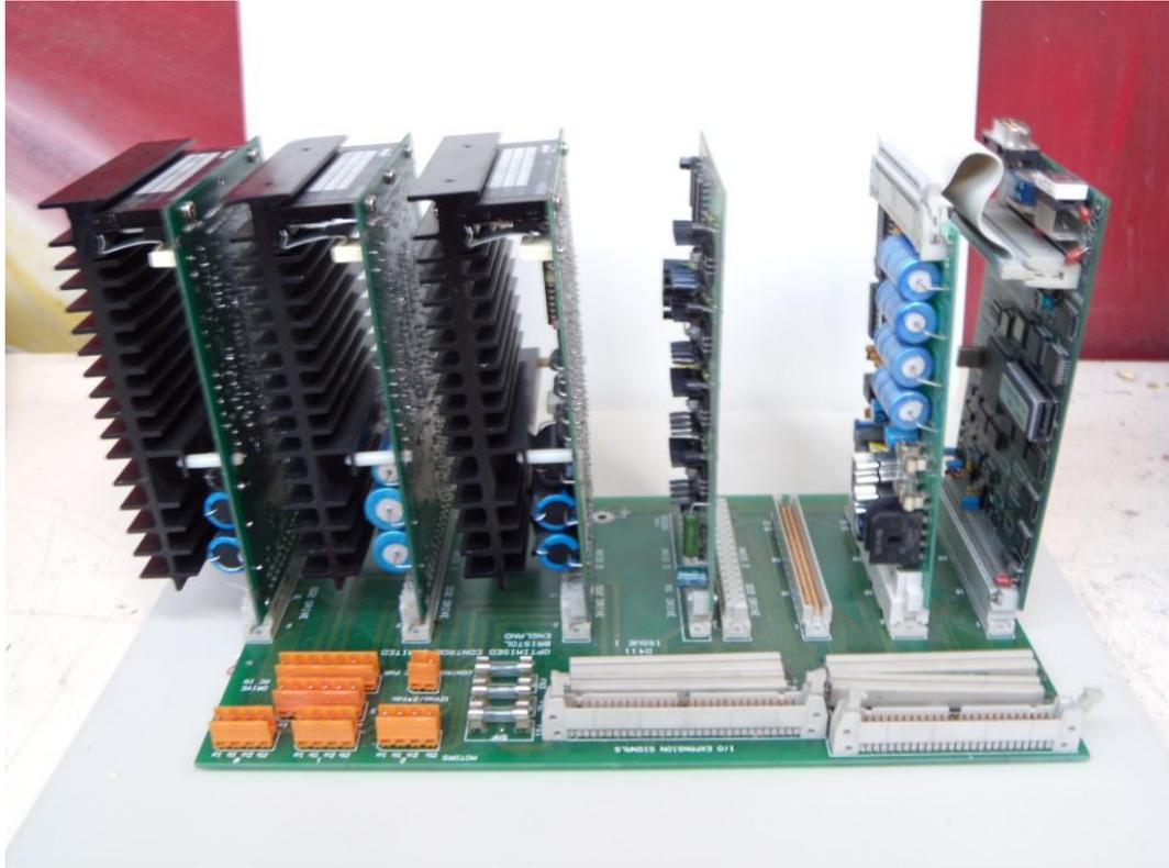
**Figure 5.3** STARMILL-ATC motor drive system
