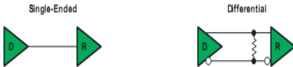
Figure 3.4 Point-to-point connection [81]
