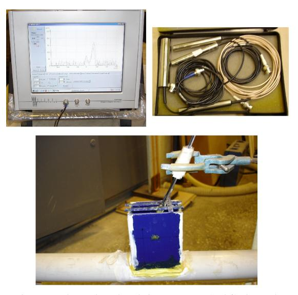
Figure 5.2.1: Ultrasound Doppler Velocimeter-DOP 2125 (top left), ultrasound probes and ultrasonic coupling condom on pipe (bottom).
