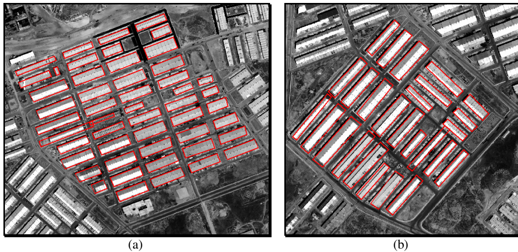
Figure 5. 17. The delineated rectangular building boundaries using Hough transform based approach for industrial areas; (a) industrial area 1 and (b) industrial area 2.
