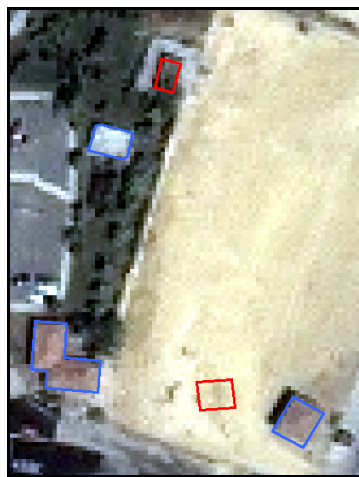
Figure 6. 2. The boundaries of destroyed and existing buildings are represented in red and blue colors, respectively.
