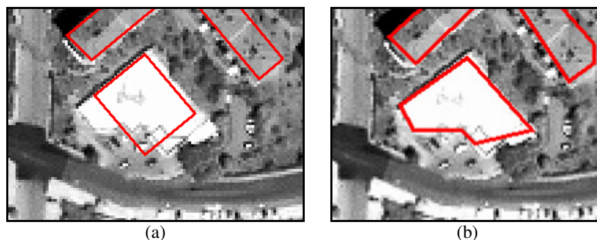
Figure 5. 25. The results of delineating a building using (a) the Hough transform based approach and (b) the Boundary tracing based approach.
