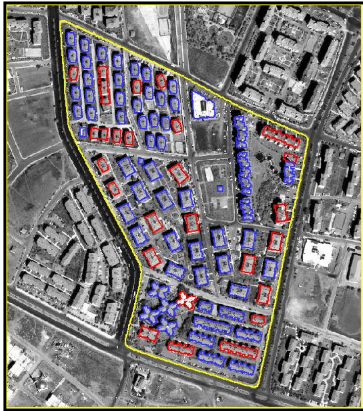
Figure 6. 12. The updated building boundaries. The blue polygons represent the existing building boundaries, while the red polygons illustrate the updated building boundaries.
