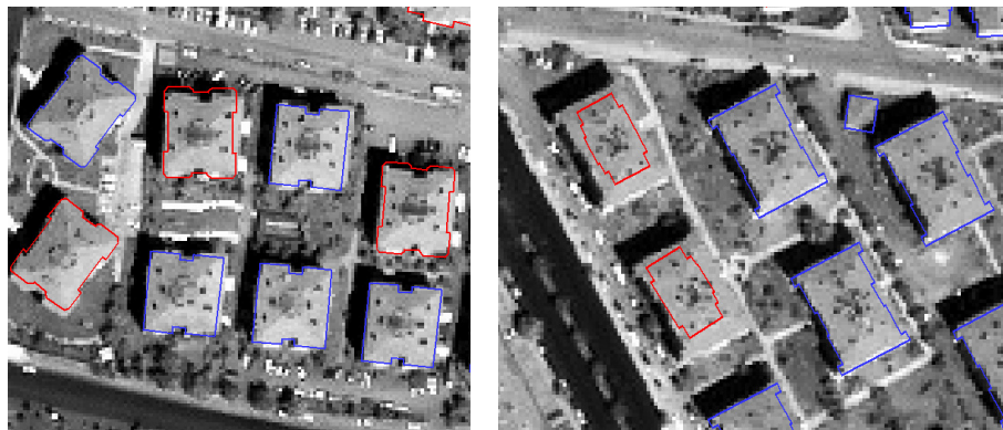
Figure 6. 16. The delineated building boundaries. Because of the similar shape parameters the building models can be selected erroneously.
