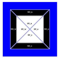
(a) A view of the predator architecture. The big square represents the body of a predator. The triangles refer to 4 directional predator sensors and 4 directional prey sensors. For each direction, each prey and predator sensor pair is designed to be overlapped. SY denotes a prey sensor, whereas SD is a predator sensor. n, s, e, and w refer to north, south, east, and west directions, respectively.
