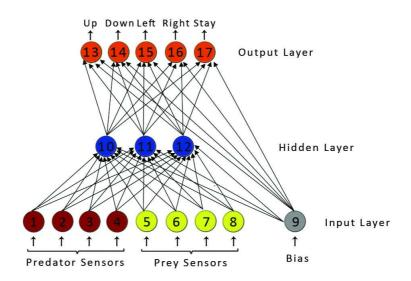
Figure 3.3: The architecture of the neural network controller. 9 input neurons (1-4: predator sensors, 5-8: prey sensors, 9: bias), 3 hidden neurons, and 5 output neurons (1:up, 2: down, 3:left, 4:right, 5:stay) are shown. First 8 input neurons are connected to hidden ones, whereas bias is connected to both hidden and output neurons.
