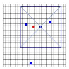
(b) A predator with its square-shaped field of vision. *P* denotes the said predator. The diagonal lines are used to differentiate the sensing fields of directional sensors.
