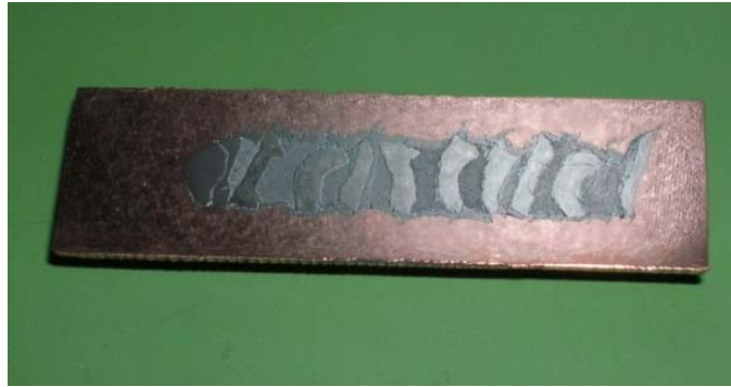
Figure 4. 3 Photograph of longitudinal section of a Cu block with embedded layers of Mg-Ni
