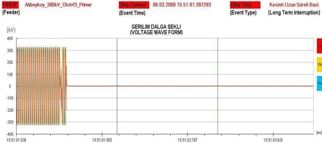
(a) Voltage – Time Graph of the Raw Data of the Voltage Interruption Event
