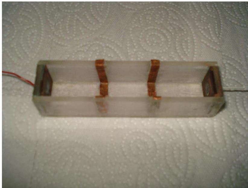
Figure A.7 Conductivity Cell
