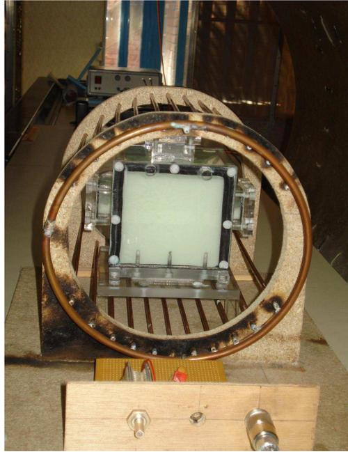
Figure A.2 RF coil with the phantom inside.
