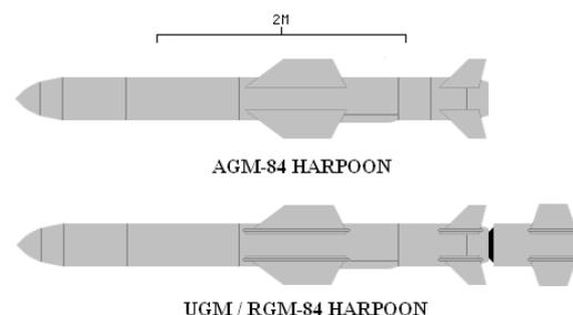
Figure 7.1 Harpoon with Booster and without Booster [24]
