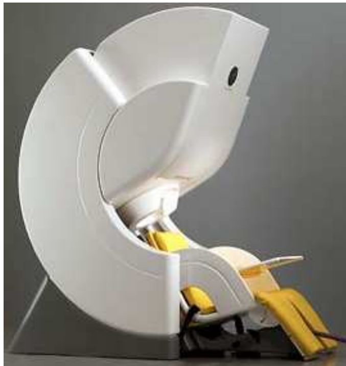
Figure 2-5 : The picture of a Magnetoencephalographm. Due to the size of the instrumentation, MEG systems are impractical in BCI applications for daily use [58].
