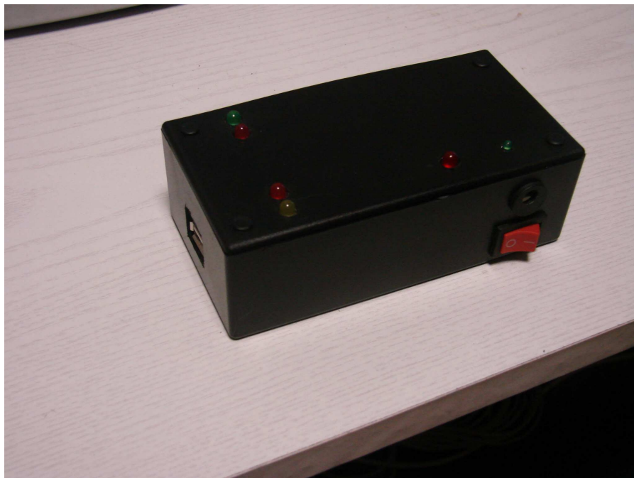
Figure B - 9: Pictures of the digitizing system. The analog signals are digitized by A/D conversion and sent to the computer via USB.
