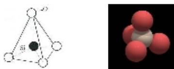
**Figure 2** Three-dimensional Si-O tetrahedron (The solid dot represents silicon; the open circles are oxygen atoms around silicon (Le Bourhis, 1997). Each oxygen atom has the same distance to the silicon atom, and the distances between the oxygen atoms are also all the same) (source: [www.quartzpage.de/gen\\_struct.html](http://www.quartzpage.de/gen_struct.html), last visited on August 2009)
