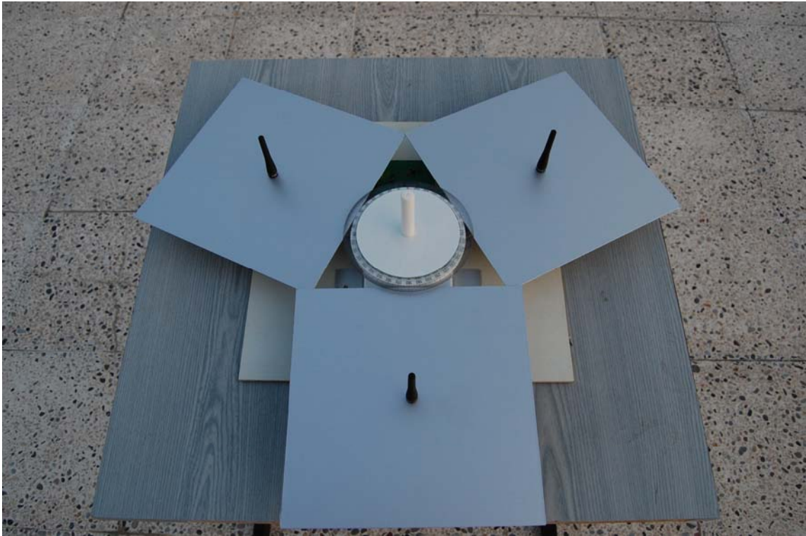
Figure 5.2 – Three Antenna DF System with Angle Measurement Apparatus
