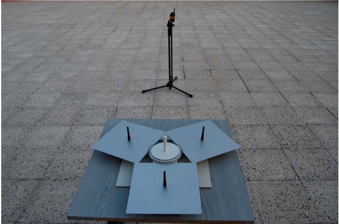
Figure 5.3 – Three Antenna Direction Finding System and Signal Transmitter
