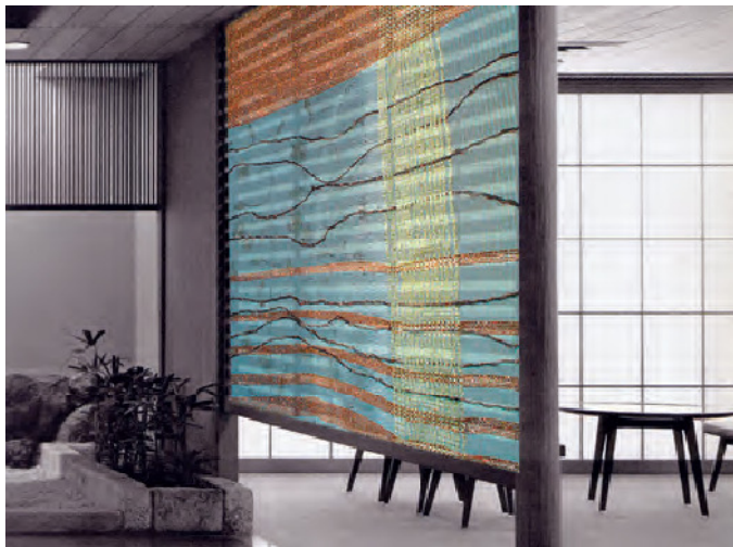
Figure 2.6.b. Shape memory interior textiles using SMA threads. (Ritter 2007)
