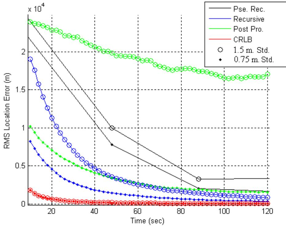
Figure 6.21: RMS Location Error with sensor location uncertainty of standard deviations 0.75 and 1.5 m. for Emitter #2.
