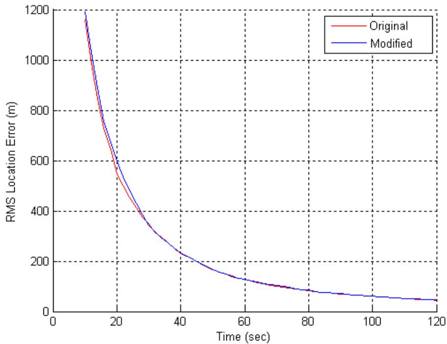
Figure 6.3: The RMS location error for non-manoevring case for Emitter #2.
