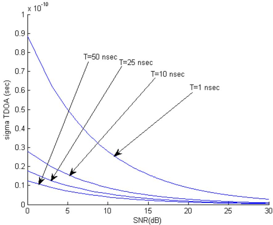
Figure 2.3: Effect of SNR, integration time and frequency on TDOA estimation for high SNR case.
