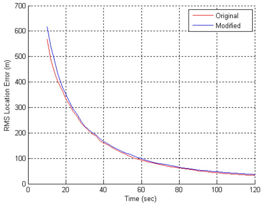
Figure 6.2: The RMS location error for non manoeuvring case for Emitter #1.
