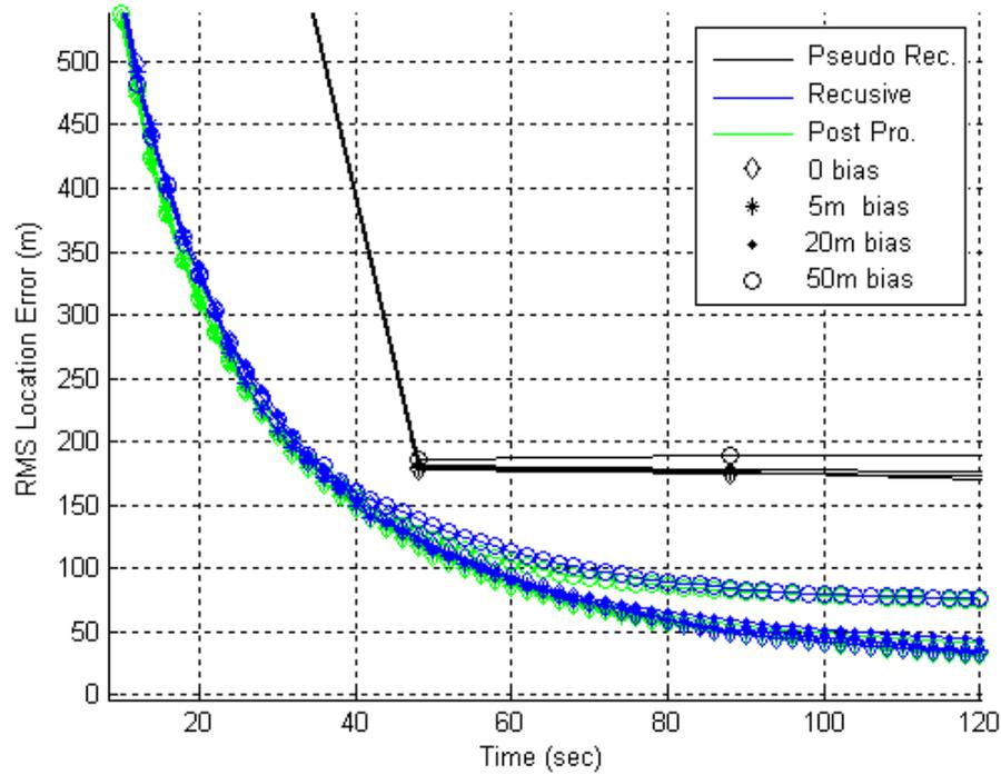
Figure 6.22: The simulation results for biased sensor locations for Emitter #1.
