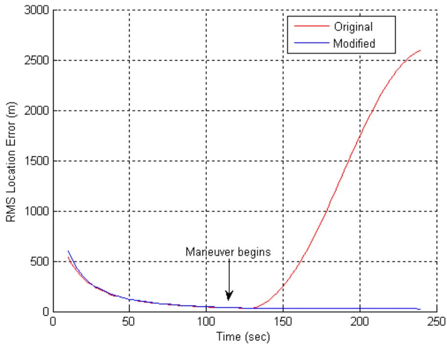
Figure 6.4: The RMS location error for the manoeuvring case for Emitter #1.
