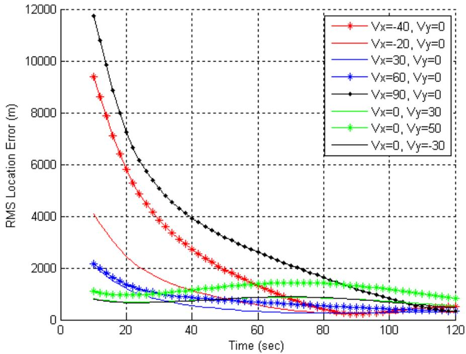
Figure 6.8: The track estimation of a moving source for Emitter #1.
