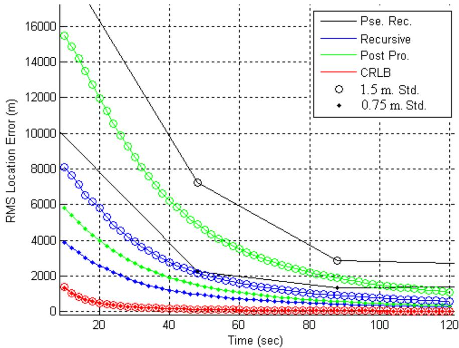
Figure 6.20: RMS Location Error with sensor location uncertainty of standard deviations 0.75 and 1.5 m. for Emitter #1.
