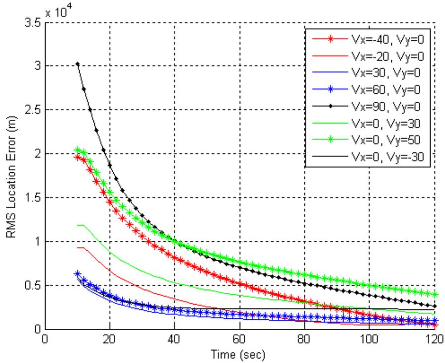
Figure 6.9: The track estimation of a moving source for Emitter #2.
