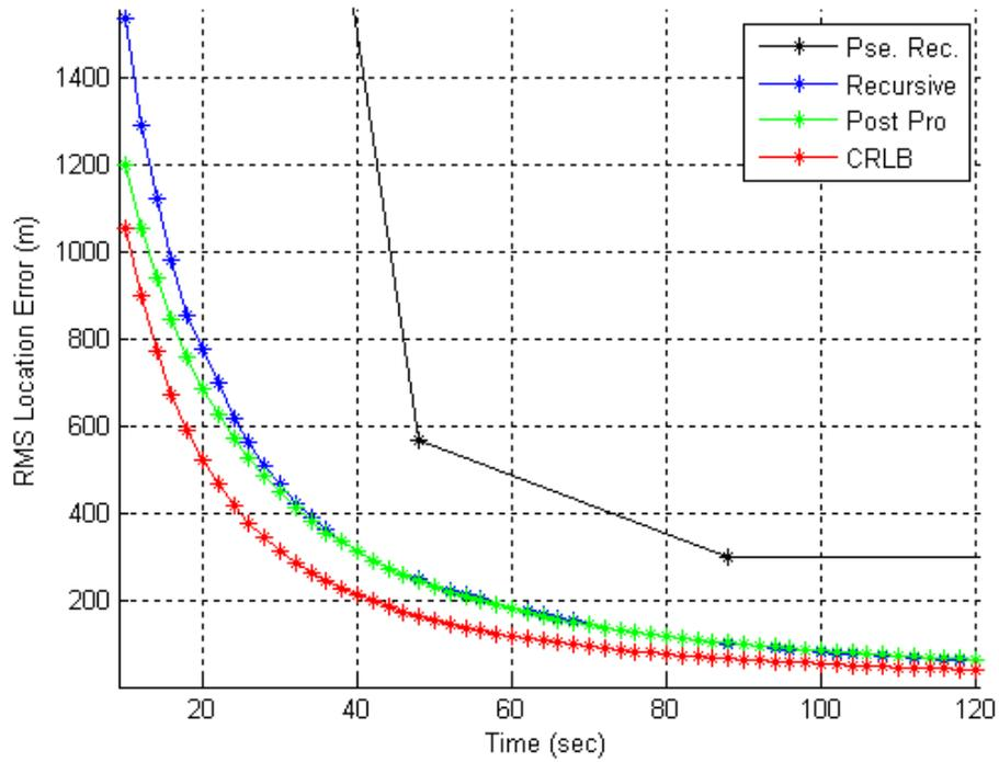
Figure 6.19: RMS Location Error with sensor location uncertainty of standard deviation 0.1 m. for Emitter #2.
