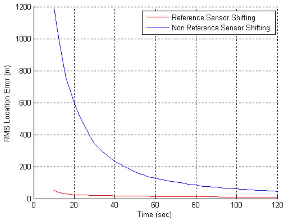
Figure 6.7: The RMS location error with the Reference Sensor Shifting for Emitter #2.
