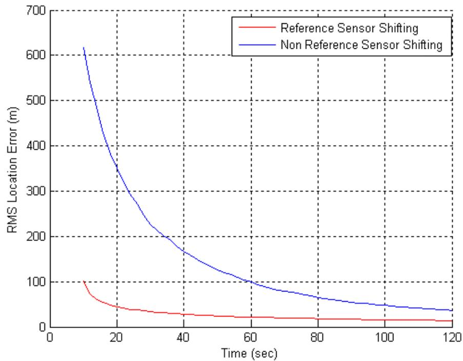
Figure 6.6: The RMS location error with the Reference Sensor Shifting for Emitter #1.
