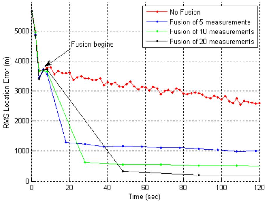
Figure 6.13: Convergence delay avoidance study for Emitter #2.
