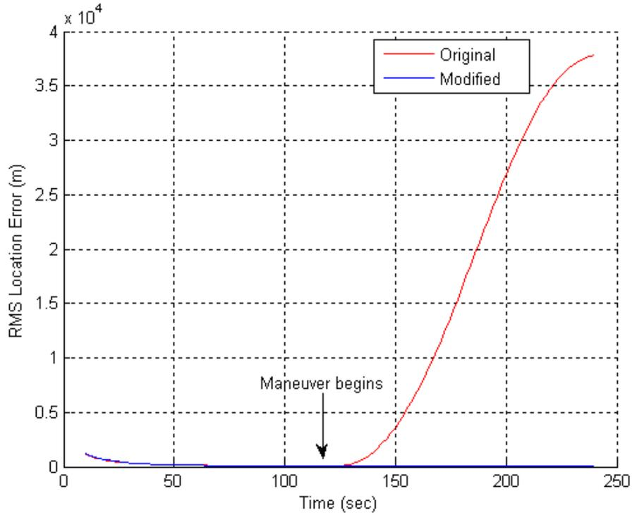
Figure 6.5: The RMS location error for manoeuvring sensor case for Emitter #2.
