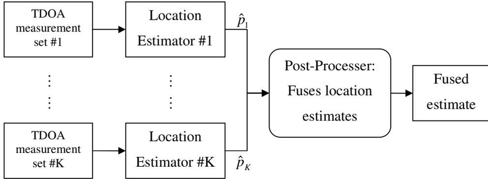
Figure 3.1: Concept of post-processing method
