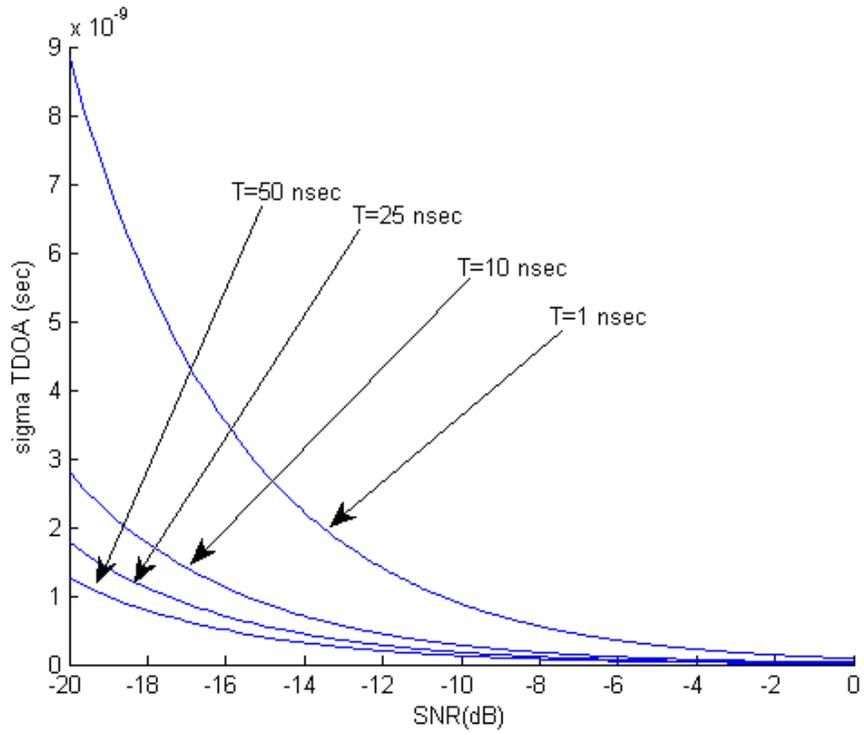
Figure 2.2: Effect of SNR, integration time and frequency on TDOA estimation for low SNR case.
