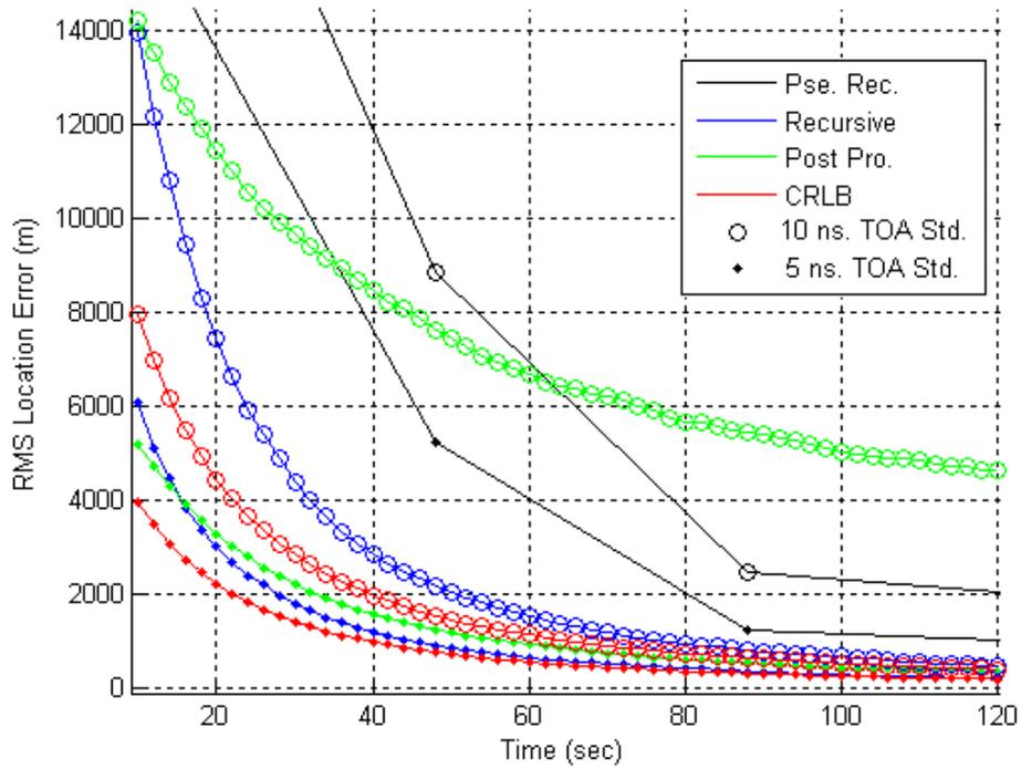
Figure 6.17: Simulation results with 5 and 10 nsec TOA noise standard deviation for Emitter #2.
