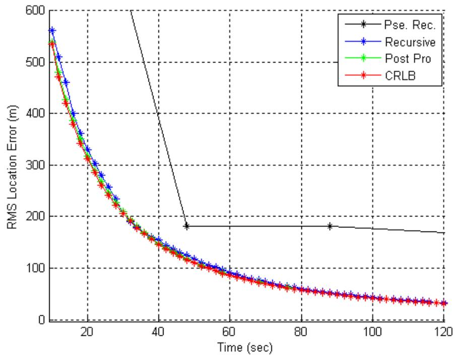
Figure 6.14: Simulation results with 1 nsec standard deviation for Emitter #1.
