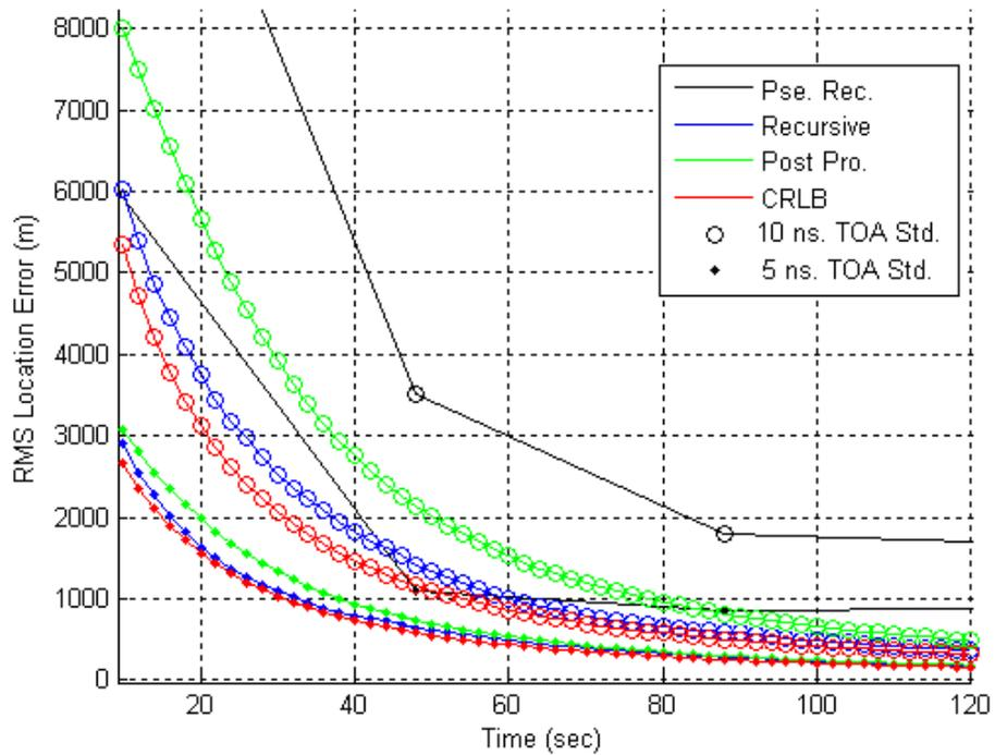
Figure 6.16: Simulation results with 5 and 10 nsec TOA noise standard deviation for Emitter #1.
