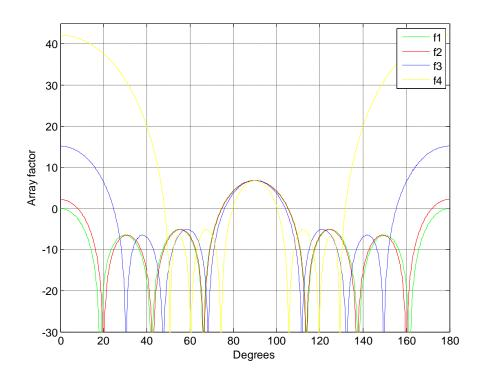
Figure - 7. 6: Array factor (dB) for %1, %10, %50 frequency changes for 7-element array
