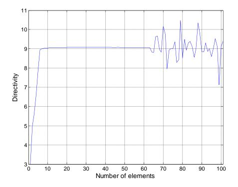
Figure - 3.5: Directivity vs Number of elements obtained by using pinv()
