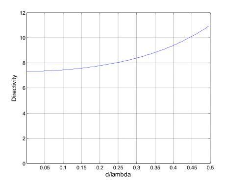
Figure - 4. 10: Directivity vs spacing for 11-element array
