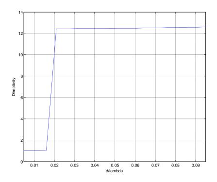
Figure - 4. 18: Directivity vs spacing for 19-element array
