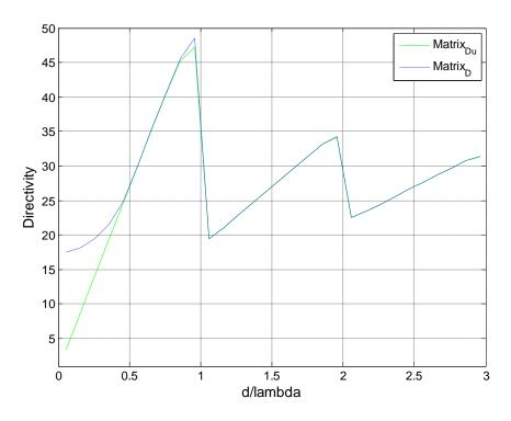
Figure - 5. 25: Directivites vs spacing for 27-element array
