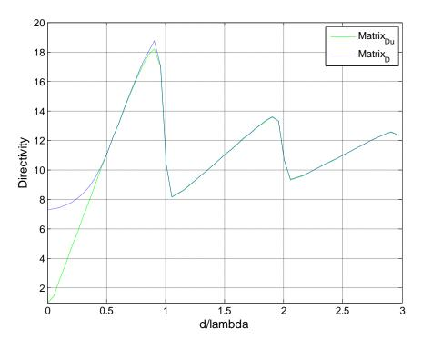
Figure - 5. 9: Directivites vs spacing for 11-element array
