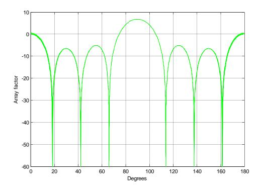
Figure - 7. 7: Array factor (dB) for smaller than 0.3% frequency change for 7-element array
