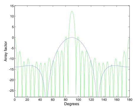
Figure - 5. 26: Array factors (dB) for 27-element array
