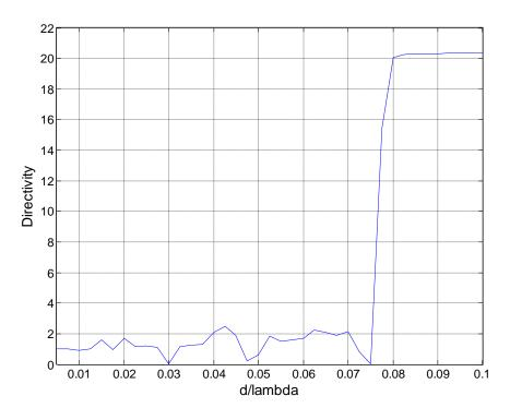
Figure - 4. 30: Directivity vs spacing for 31-element array
