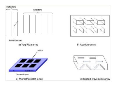
Figure - 2. 1: Typical wire, aperture and microstrip array configurations
