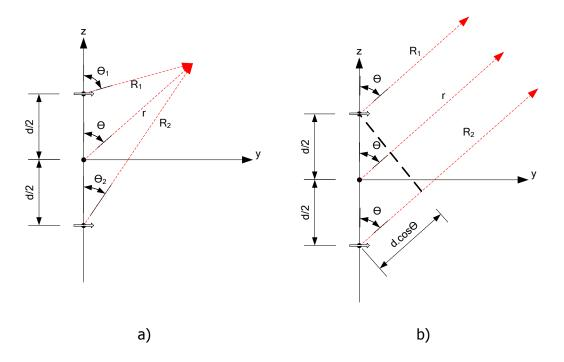
Figure - 2. 2: a) Two infinitesimal dipoles, b) Far-field observations
