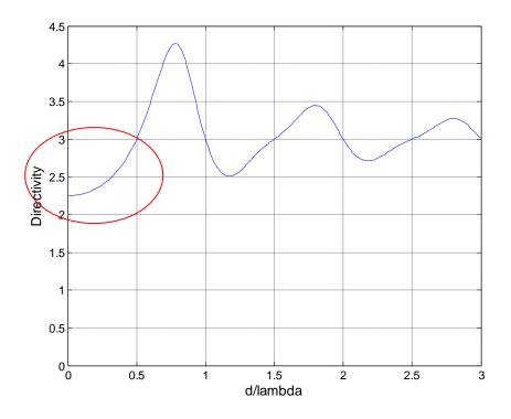
Figure - 4. 1: Directivity versus distance between the elements for 3-element array
