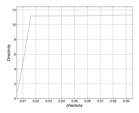
Figure - 4. 16: Directivity vs spacing for 17-element array
