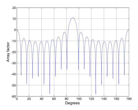
Figure - 4. 19: Array factor (dB) for 19-element superdirective array
