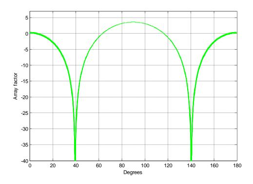
Figure - 7. 3: Array factor (dB) for smaller than 1% frequency change for 3-element array
