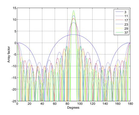
Figure - 4. 40: Array factors (dB) for 3,11,17,23,29 and 37 elements
