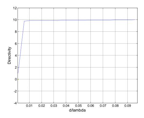
Figure - 4. 14: Directivity vs spacing for 15-element array
