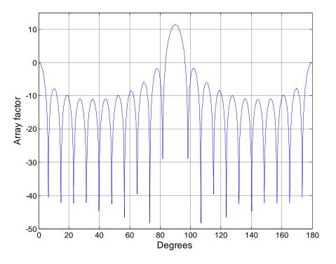
Figure - 4. 21: Array factor (dB) for 21-element superdirective array
