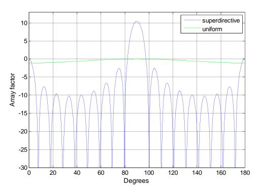
Figure - 5. 16: Array factors (dB) for 17-element array
