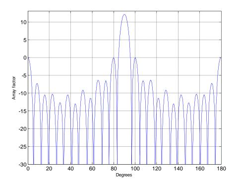
Figure - 4. 25: Array factor (dB) for 25-element superdirective array
