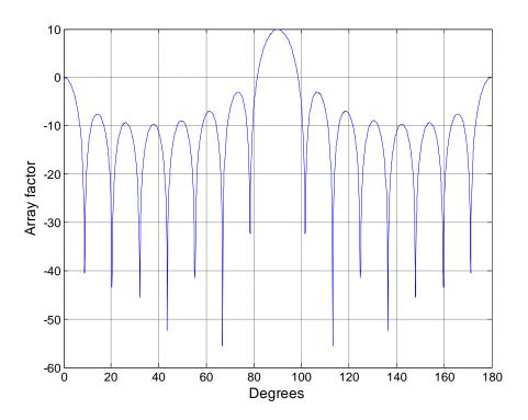
Figure - 4. 15: Array factor (dB) for 15-element superdirective array
