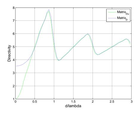
**Figure - 5. 3:** Directivity versus spacing for 5-element array (Dashed curve represents stationary directivity, solid line represents uniform directivity)
