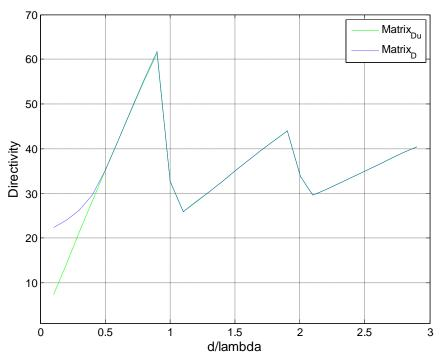
Figure - 5. 33: Directivities vs spacing for 35-element array
