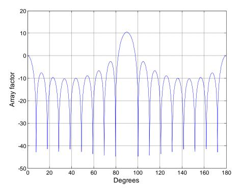
Figure - 4. 17: Array factor (dB) for 17-element superdirective array
