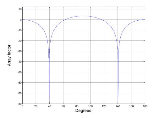
Figure - 4. 3: Array factor (dB) for 3-element superdirective array
