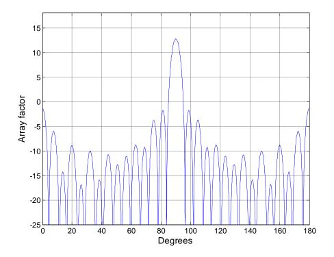
Figure - 4. 29: Array factor (dB) for 29-element superdirective array
