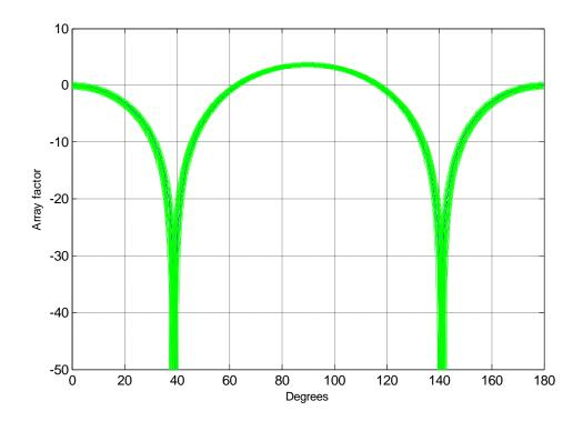
Figure - 6. 3: Perturbated Array factors (dB) for 3-element array
