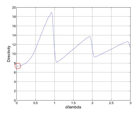
**Figure - 3.14:** Direcitivy vs  $d/\lambda$  for number of elements 11 obtained by using mp toolbox
