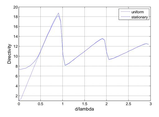
Figure - 3.15: Stationary and uniform directivity curves for 11 elements
