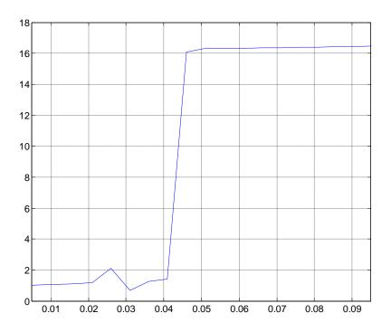
Figure - 4. 24: Directivity vs spacing for 25-element array
