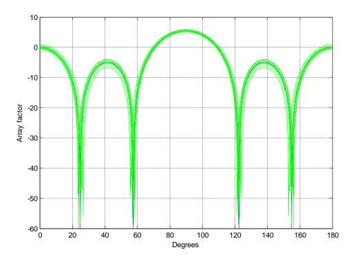
Figure - 6. 4: Perturbated Array factors (dB) for 3-element array
