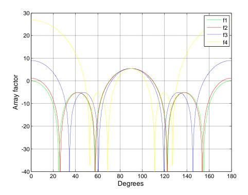
Figure - 7. 4: Array factor (dB) for %1, %10, %50 frequency changes for 5-element array
