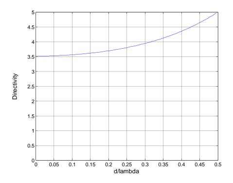
Figure - 4. 4: Directivity vs spacing for 5-element array
