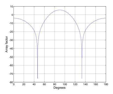
Figure - 3.3: Array factor (dB) for 73 elements
