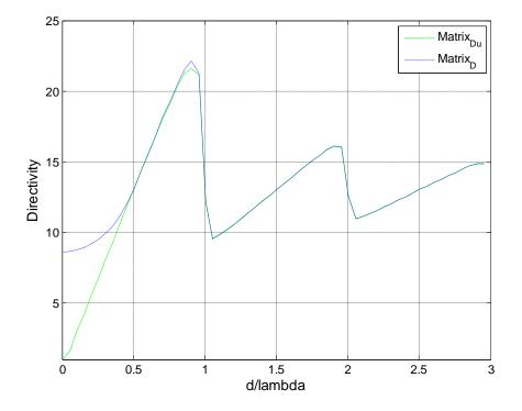
Figure - 5. 11: Directivities vs spacing for 13-element array
