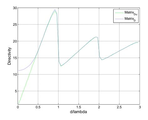
**Figure - 5. 15:** Directivities vs spacing for 17-element array (Dashed curve represents stationary directivity, solid line represents uniform directivity)
