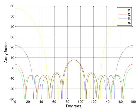
Figure - 7.8: Array factor (dB) for %1, %10, %50 frequency changes for 7-element array
