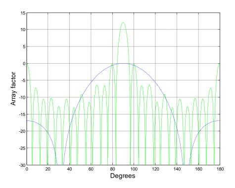
Figure - 5. 24: Array factors (dB) for 25-element array
