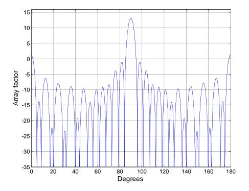
Figure - 4. 31: Array factor (dB) for 31-element superdirective array
