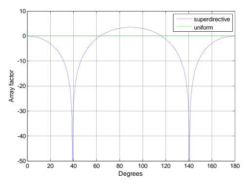
Figure - 5. 2: Array factors (dB) for 3-element array
