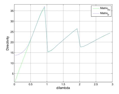
Figure - 5. 19: Directivites vs spacing for 21-element array
