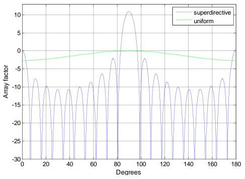
Figure - 5. 18: Array factors (dB) for 19-element array
