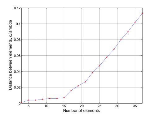
Figure - 4. 39: Minimum spacing for accurate calculations vs Number of elements
