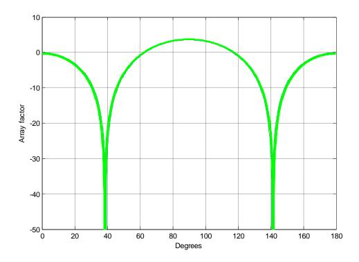
Figure - 6. 2: Perturbated Array factors (dB) for 3-element array
