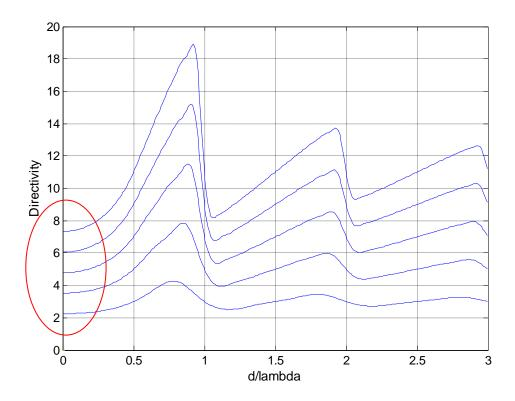
**Figure - 5. 38:** Directivity vs spacing for 3, 5, 7, 9 and 11 elements (The bottom curve is for 3-element case and the top is for 11 elements)
