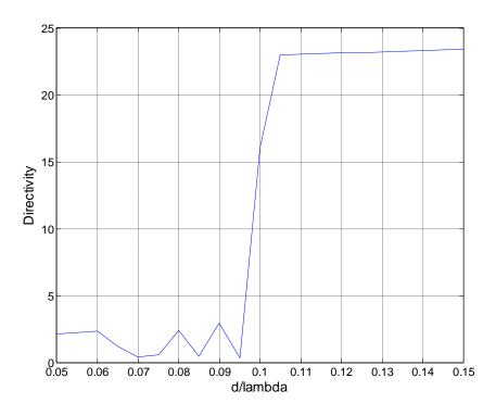
Figure - 4. 36: Directivity vs spacing for 37-element array
