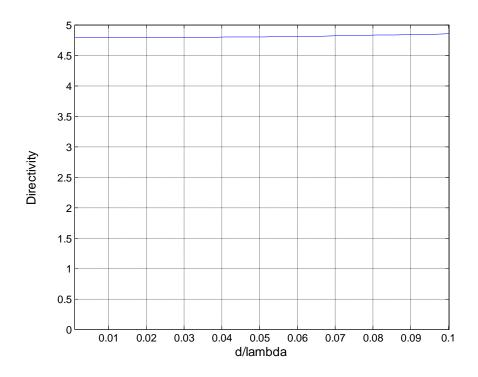
Figure - 4. 6: Directivity vs spacing for 7-element array
