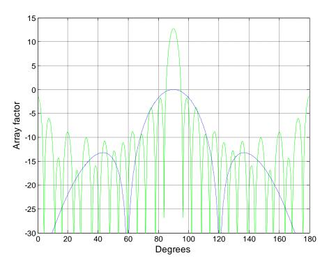
Figure - 5. 28: Array factors for 29-element array
