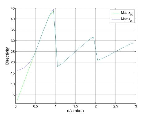
Figure - 5. 23: Directivities vs spacing for 25-element array
