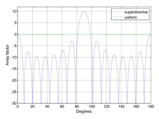
Figure - 5. 14: Array factors (dB) for 15-element array
