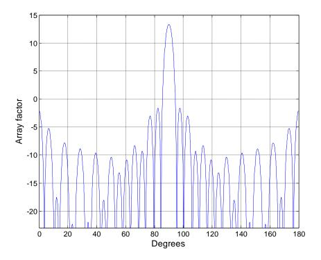
Figure - 4. 35: Array factor (dB) for 35-element superdirective array
