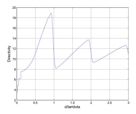
Figure - 3.11: Direcitivy vs d/ $\lambda$  for number of elements 11 obtained by using pinv()
