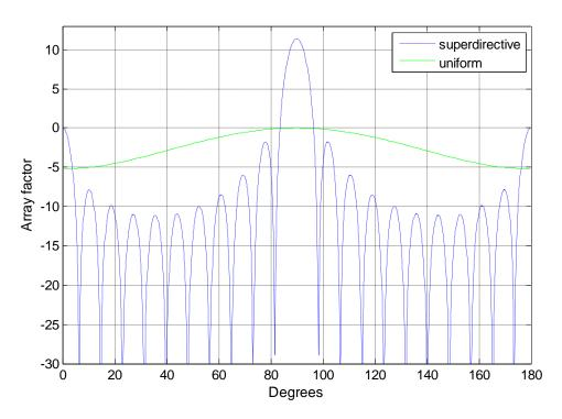
Figure - 5. 20: Array factors (dB) for 21-element array
