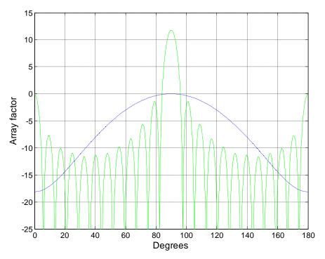
Figure - 5. 22: Array factors (dB) for 23-element array
