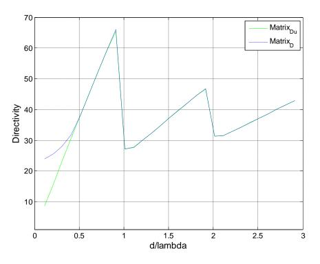
Figure - 5. 35: Directivities vs spacing for 37-element array
