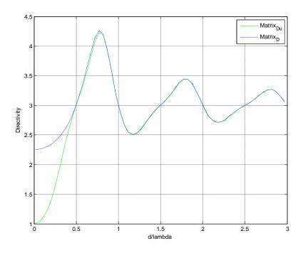
Figure - 5. 1: Directivity vs spacing for 3-element array
