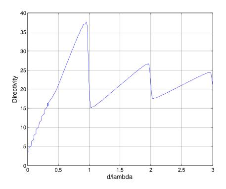
**Figure - 3.13:** Direcitivy vs  $d/\lambda$  for number of elements 11 obtained by using bicg()
