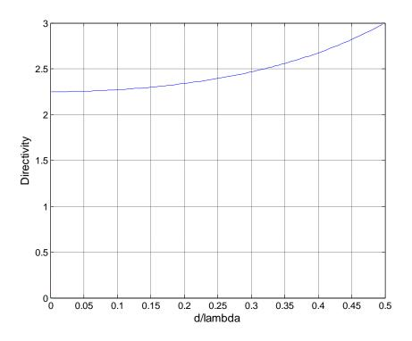
Figure - 4. 2: Directivity vs spacing for 3-element array
