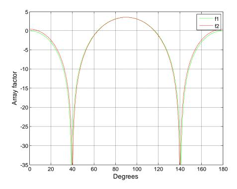
Figure - 7. 1: Array factor (dB) for 1% frequency change for 3-element array
