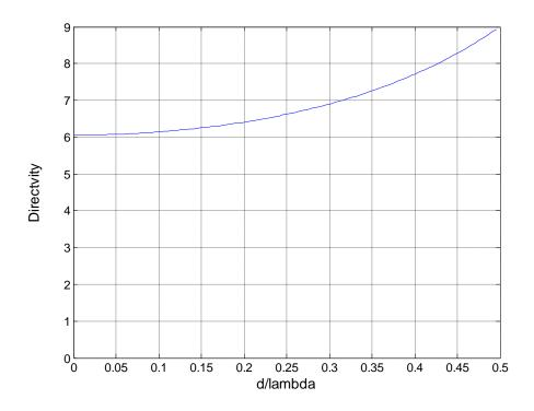
Figure - 4. 8: Directivity vs spacing for 9-element array
