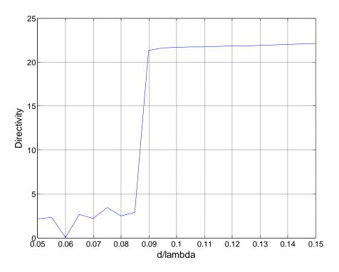
Figure - 4. 32: Directivity vs spacing for 33-element array
