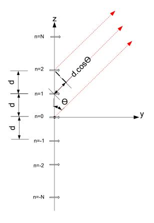
Figure - 3. 1: Array of 2N+1 elements lying on z axis
