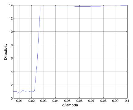
Figure - 4. 20: Directivity vs spacing for 21-element array
