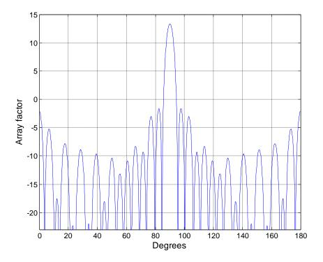
Figure - 4. 33: Array factor (dB) for 33-element superdirective array
