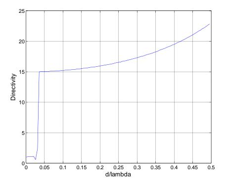
Figure - 4. 22: Directivity vs spacing for 23-element array
