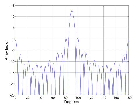
Figure - 4. 27: Array factor (dB) for 27-element superdirective array
