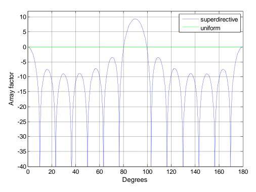
Figure - 5. 12: Array factors (dB) for 13-element array
