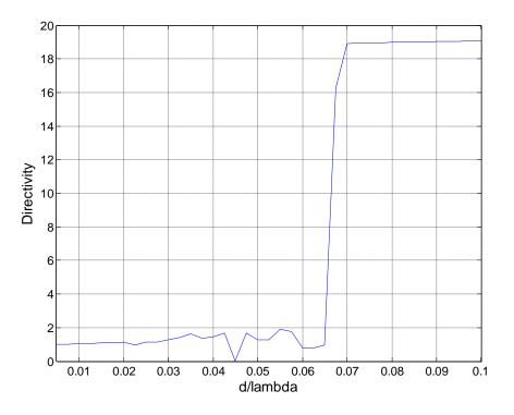
Figure - 4. 28: Directivity vs spacing for 29-element array
