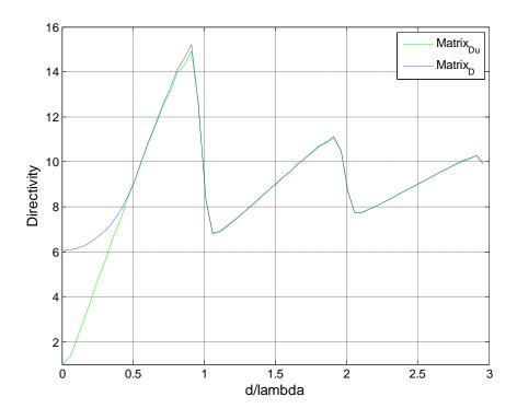
Figure - 5. 7: Directivities vs spacing for 9-element array
