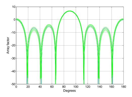
Figure - 6. 5: Perturbated Array factors (dB) for 7-element array
