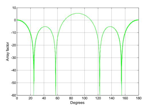
Figure - 7. 5: Array factor (dB) for smaller than 0.5% frequency change for 5-element array
