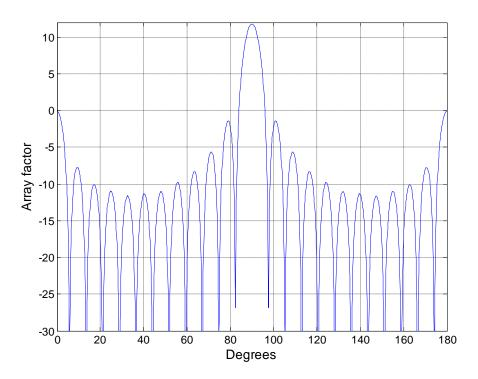
Figure - 4. 23: Array factor (dB) for 23-element superdirective array
