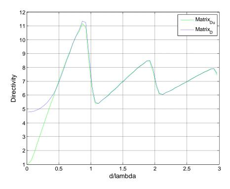
Figure - 5. 5: Directivities vs spacing for 7-element array
