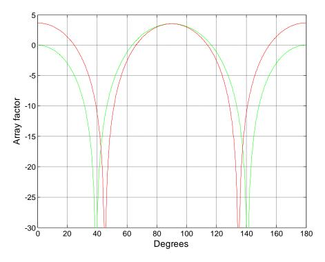
Figure - 7. 2: Array factor (dB) for 10% frequency change for 3-element array
