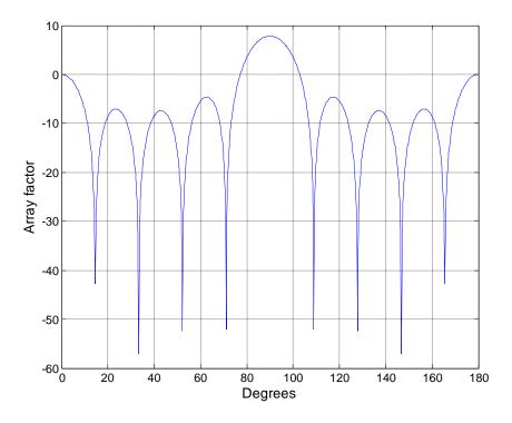
Figure - 4. 9: Array factor (dB) for 9-element superdirective array
