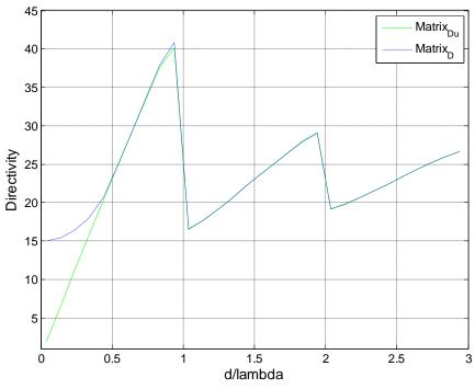
Figure - 5. 21: Directivites vs spacing for 23-element array
