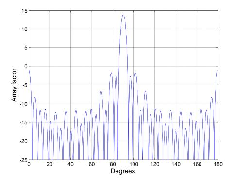
Figure - 4. 37: Array factor (dB) for 37-element superdirective array
