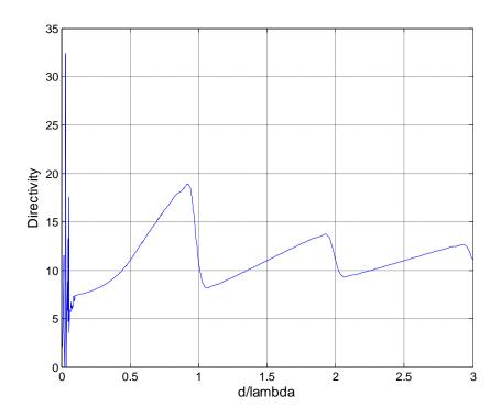
Figure - 3.10: Direcitivy vs d/ $\lambda$  for number of elements 11 obtained by using inv()
