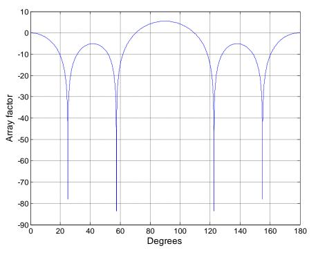
Figure - 4. 5: Array factor (dB) for 5-element superdirective array
