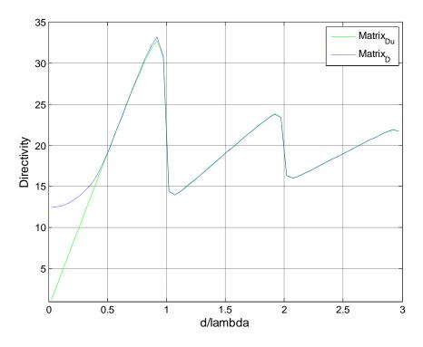
Figure - 5. 17: Directivites vs spacing for 19-element array
