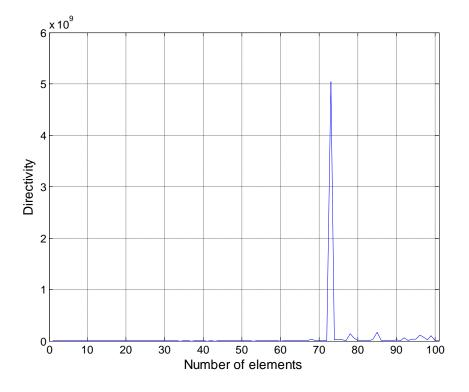
Figure - 3.2: Directivity vs Number of elements for fixed array length
