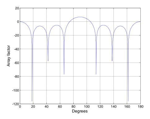
Figure - 4. 7: Array factor (dB) for 7-element superdirective array
