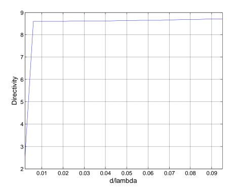
Figure - 4. 12: Directivity vs spacing for 13-element array
