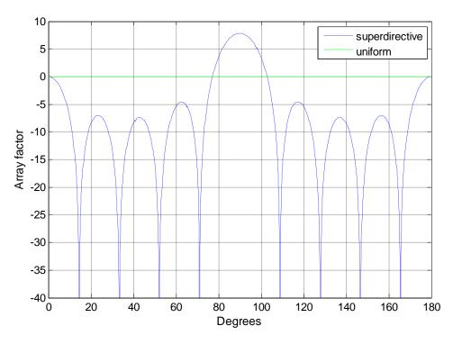
Figure - 5. 8: Array factors (dB) for 9-element array
