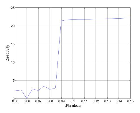
Figure - 4. 34: Directivity vs spacing for 35-element array
