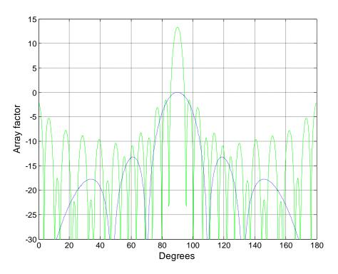
Figure - 5. 32: Array factors for 33-element array
