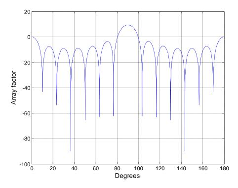
Figure - 4. 13: Array factor (dB) for 13-element superdirective array
