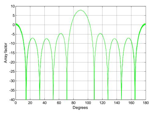
Figure - 7. 9: Array factor (dB) for smaller than 0.1% frequency change for 9-element array
