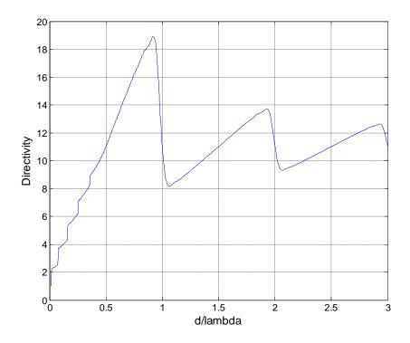
**Figure - 3.12:** Direcitivy vs  $d/\lambda$  for number of elements 11 obtained by using pinv( ,1e-3)
