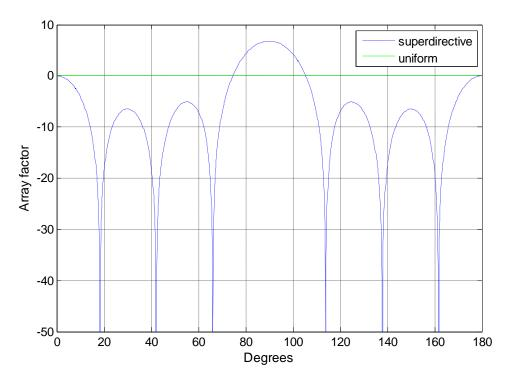
Figure - 5. 6: Array factors (dB) for 7-element array
