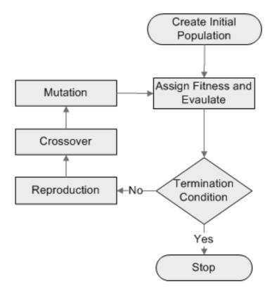
Figure 3 Working Principle of a Generic GA
