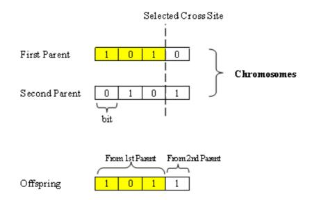
Figure 22 Generation of the offspring by single point crossover operator
