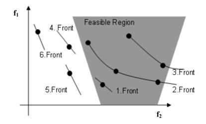
Figure 4 Determining Fronts in NSGA-II with Constraint Tournament Method
