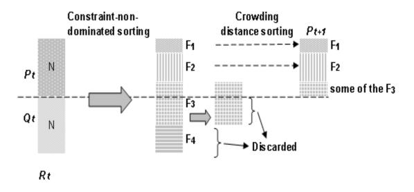
Figure 6 Schema of the NSGA-II with Constraint Tournament Method
