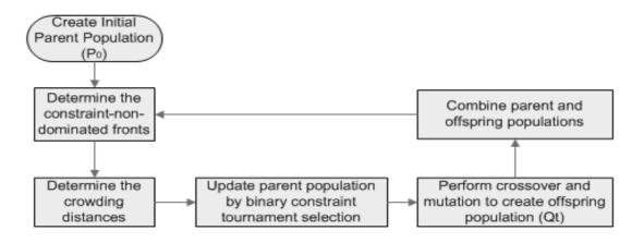
Figure 7 Steps of the NSGA-II with constraint tournament method
