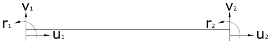
Figure 2.2-5 Degrees of freedom of a frame member
