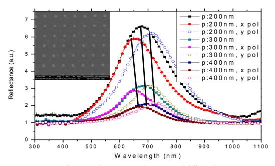
Figure 5.22: Reflectance of Ag nanoparticle arrays with different lattice constants. Polarized components of the peaks are also given. Inset presents the SEM image of corresponding Ag nanoparticles.
