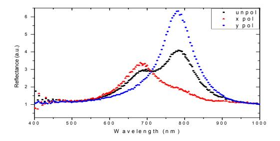
*Figure 5.15: Reflectance spectra of ellipsoidal Au nanoparticles with lattice constant of 400 nm.*
