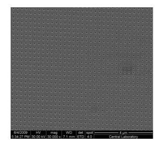
Figure 4.5: Array of nanoholes patterned on PMMA over an ITO coated microscope slide. 100 nm diameter holes with a period of 300 nm will serve as a mask in further steps.
