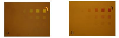
Figure 5.28: Images of Ag nanoparticle arrays with varying lattice parameters and particle diameters, taken through optical microscope under front (a) and back (b) illumination.
