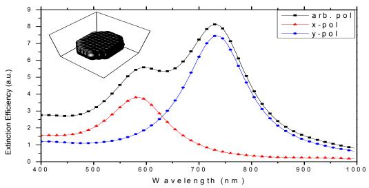
Figure 5.6: DDA simulation of Au ellipsoid with axes of 80-110 nm and height of 20 nm located on ITO coated glass.
