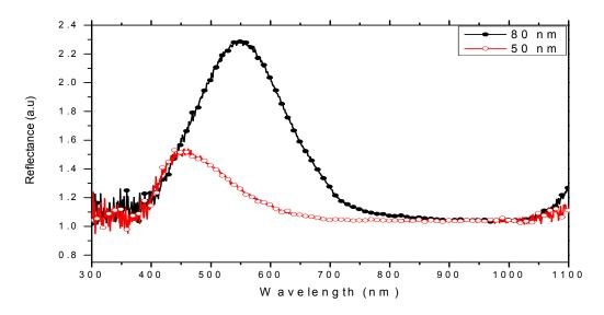
Figure 5.24: Reflectance spectra of Ag nanodisks with diameters of 50 and 80 nm.
