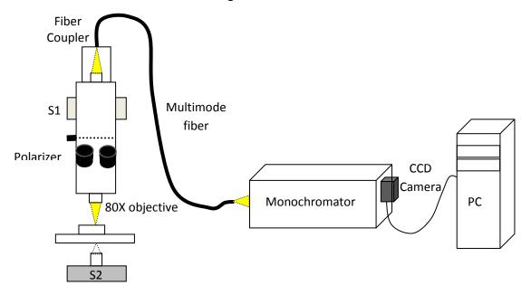
*Figure 4.16: Illustration of the optical setup used for characterization.*
