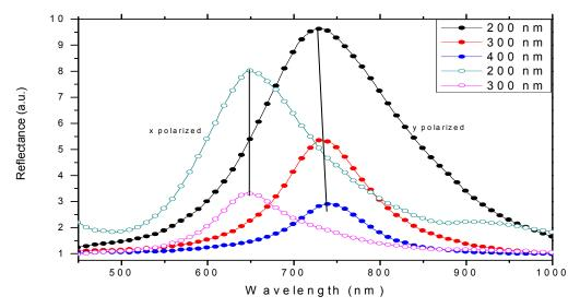
Figure 5.8: Reflectance from arrays with same nanoparticle sizes, 80-110 nm, but varying lattice constants form 200 to 400 nm.
