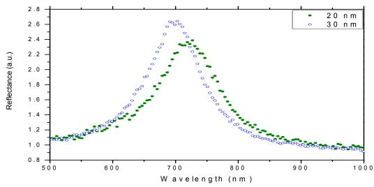
*Figure 5.11: Reflectance of Au nanoparticle arrays with all parameters kept constants except the thicknesses.*
