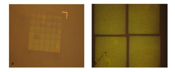
Figure 4.17: Reflection images of nanoparticle arrays with dimensions of (a) 600x600 and (b) 200x200  $\mu$ m<sup>2</sup> produced for two different optical setups described above.
