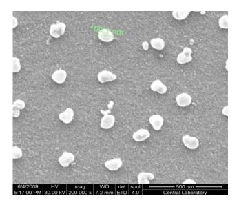
Figure 4.7: Metal nanoparticles over bare microscope slide patterned with an antistatic layer of 2 nm thick gold film. The resulting pattern is lack of symmetry because of the deviation in the path of electron beam due to charging of the sample.
