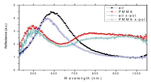
Figure 5.23: Reflectance spectra of Ag nanoparticle arrays w/o PMMA coating.
