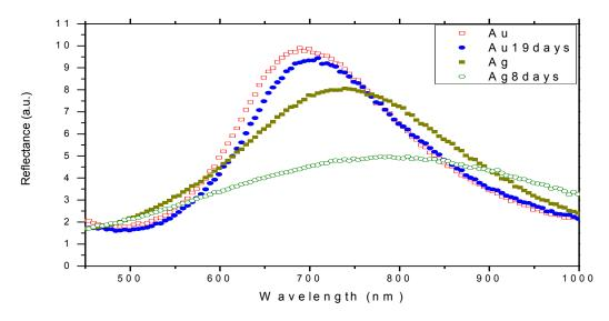
Figure 5.20: Reflectance spectra of Au and Ag nanoparticles measured multiple times.
