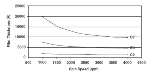
Figure 4.4: Film thicknesses obtained from different formulations of PMMA in chlorobenzene versus spin speed.
