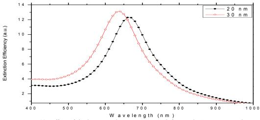
Figure 5.12: Effect of thickness on the resonance peak for single Au nanoparticles.
