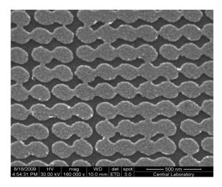
*Figure 5.14: Au ellipsoids with diameters close to the lattice parameter.*
