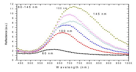
*Figure 5.4: Au nanoparticle array with a lattice constant of 200 nm patterned over ITO coated glass. Nanoparticle thicknesses are 20 nm and diameters vary between 60-145 nm.*
