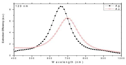
Figure 5.16: Extinction efficiency of 120 nm Au and Ag nanodisks located on ITO coated glass, simulated with DDA.
