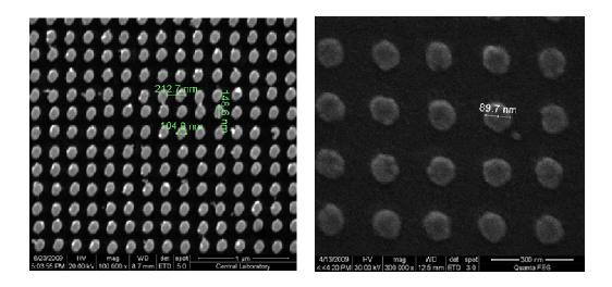
Figure 4.12: SEM images of metal nanoparticles patterned over ITO coated glass with different beam currents.
