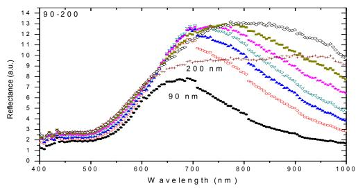
Figure 5.13: 30 nm thick ellipsoidal Au nanoparticles with varying diameters.
