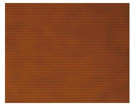
Figure 5.27: Image of an Ag nanopartcile array taken under front illumination with optical microscope. Lattice constants of the array are 200 and 1000 nm in perpendicular axes.
