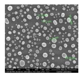
*Figure 4.2: SEM image of Au nanoparticles grown on quartz substrate with thermal evaporation followed by annealing.*
