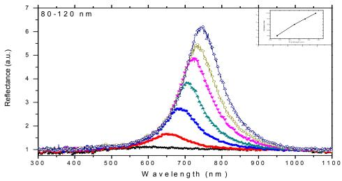
Figure 5.9: Reflectance spectra of ellipsoidal nanoparticles illuminated with polarized light with axes varying between 80-120 nm. Inset shows the dependence of peak wavelength to the particle size.
