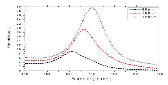
*Figure 5.10: Extinction of Au nanodisks with increasing diameters located on ITO coated glass computed with DDA simulations.*
