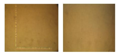
*Figure 4.8: Images of samples before development w/o heat treatment taken with optical microscope.*
