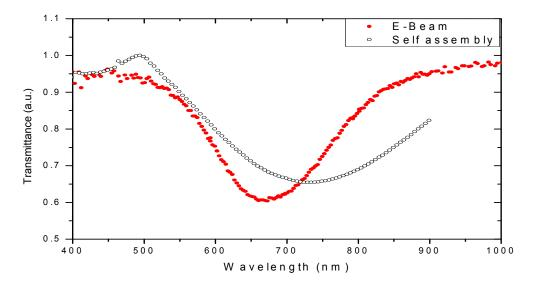
*Figure 5.1: Transmittance data of two samples produced with self assembly and electron beam lithography methods.*
