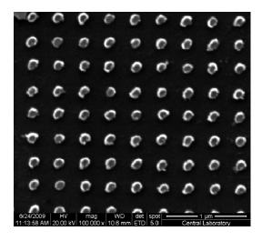
*Figure 4.9: Au particle array over glass produced by use of a thermally deposited thin Au film as antistatic layer.*
