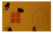
Figure 5.25: Reflection (a) and transmission (b) through Ag nanoparticles with diameters of 50 (right) and 80 (left) nm.
