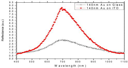
Figure 5.3: Reflectance data of Au nanoparticles patterned over glass substrates w/o ITO layer.
