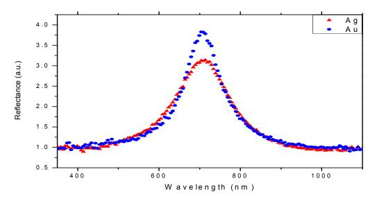
*Figure 5.19: Reflectance spectra of Au and Ag nanoparticle arrays having the same parameters.*
