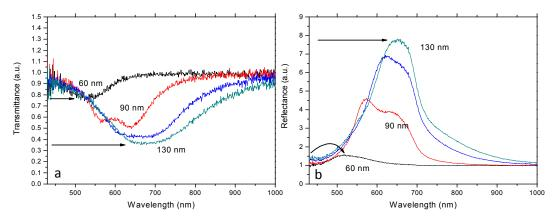
Figure 5.26: Transmittance and reflectance of Ag nanoparticles with varying size. Peak ratio of 60 and 130 nm particles in two data are found to be different.
