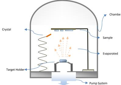
Figure 4.3: Resistive thermal evaporator system used in this work.
