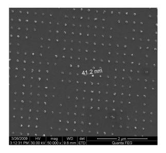
Figure 4.15: SEM image of silver nanoparticles having approximately 40 nm diameter patterned over ITO coated glass substrate.
