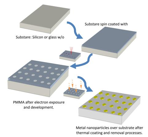
*Figure 4.6: Illustration of EBL manufacturing steps to obtain array of metal nanoparticles.*
