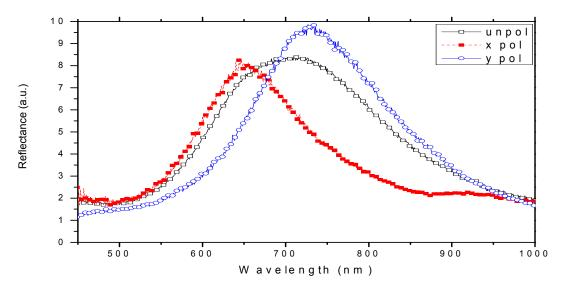
Figure 5.5: Ellipsoidal Au nanoparticles with axes 80 and 110 nm, with lattice constant of 200 nm over ITO coated glass.
