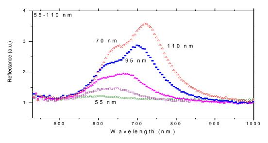
Figure 5.7: Au nanoparticle arrays with lattice constant of 300 nm. Particles are ellipsoids having dimensions varying between 55-110 nm.
