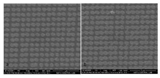
*Figure 5.18: SEM images of Ag nanoparticles with diameters of approximately 180 and 190 nm.*
