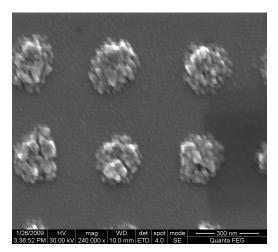
Figure 5.21: SEM image of Ag nanoparticles 30 days after the date of production.
