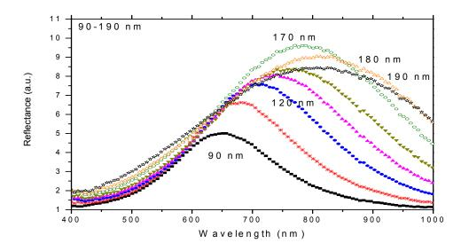
Figure 5.17: Reflectance spectra of Ag nanoparticle arrays located on ITO coated glass with a lattice constant of 200 nm. Diameters of the nanodisks vary from 90 to 190 nm.
